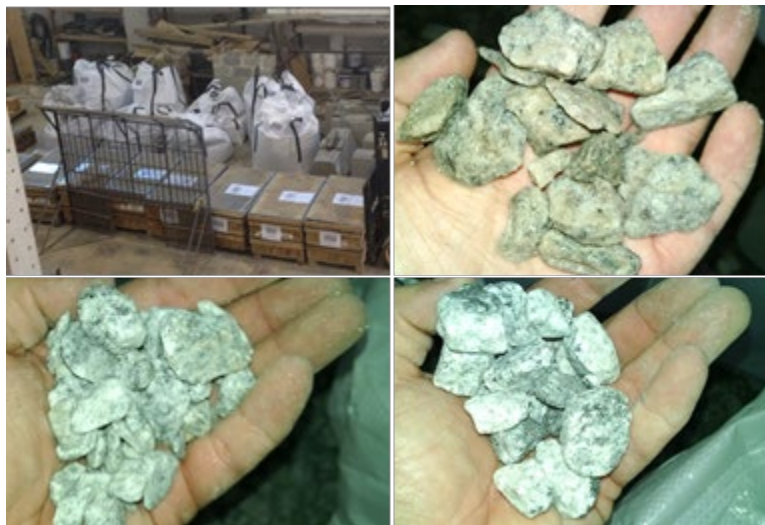
Figure 3. Weathered granite coarse aggregates: (a) as delivered to USC laboratories, (b) CA2, (c) CA3, (d) CA4
