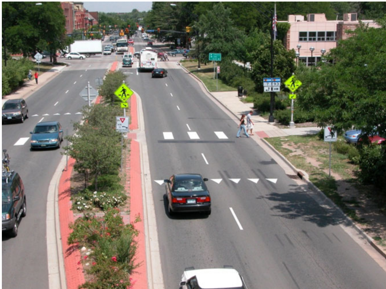
Figure 36 - Advance Yield Control Signs and Pavement Markings (Ped Bike Safe)
