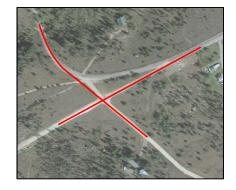
The intersection at MP 2.7 would be modified to create a standard, uncontrolled four-way intersection.
