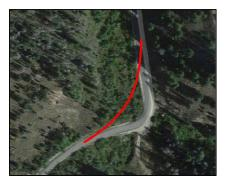
The 90-degree curve at MP 0.5 would be flattened to achieve a 40-mph design speed.
