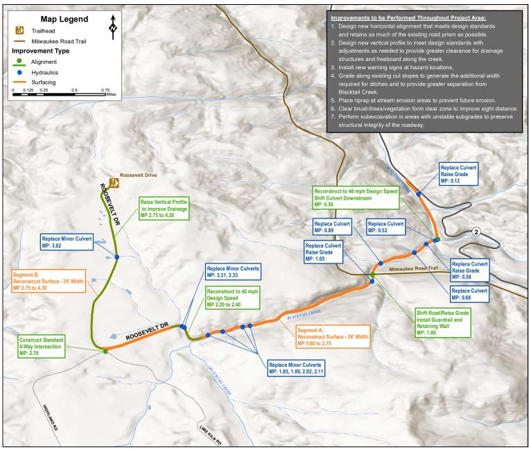
Figure 6.3: Option 3: Reconstruction with New Alignment
