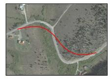
The horizontal curves on the s-curve section between MP 2.2 and 2.4 would be flattened and a consistent, increasing grade would be established.
