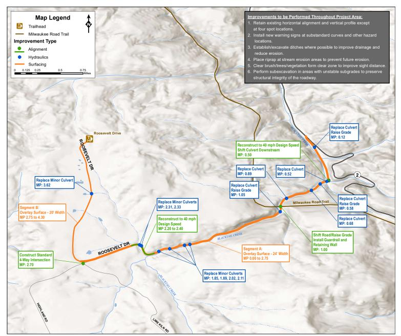
Figure 6.2: Option 2: Rehabilitation with Improved Geometrics
