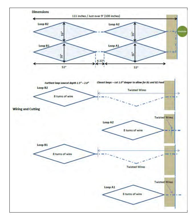
Figure 4: Inductive Loop layout
