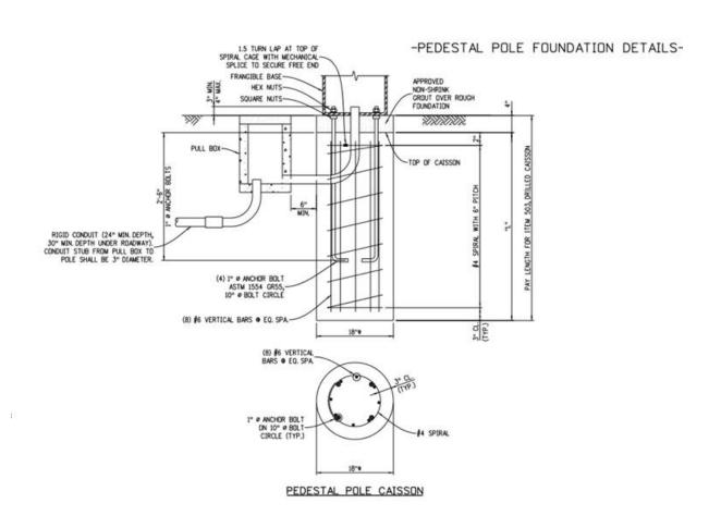
Figure 5: Sign Pedestal Pole Foundation Detail
