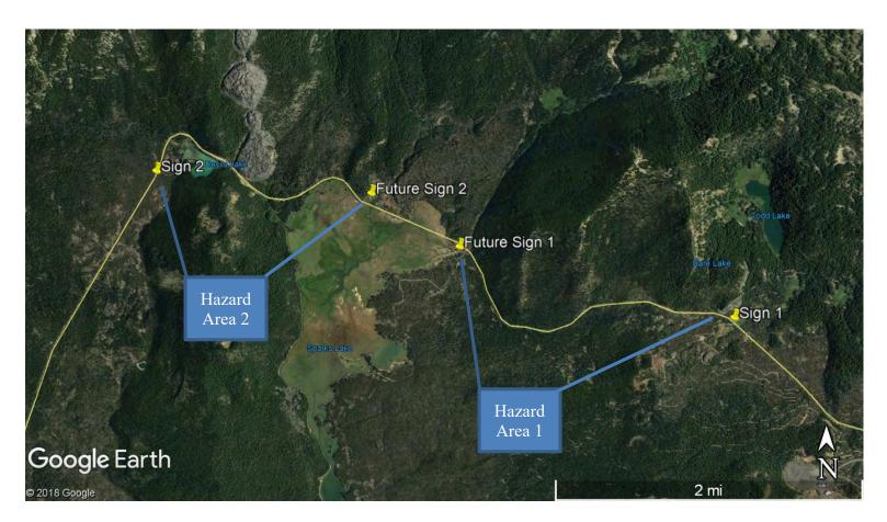
The distance between Sign 1 and Sign 2 is approximately 5 miles, and an 8-10 minute drive by car. This may be long enough for the effectiveness of the sign to fade as the motorist begins to forget the sign. It is unknown at this time what the critical time may be for when a second sign
