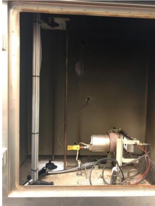
Figure 4. Laser/sensor assembly mounted in the NBS chamber adjacent to the photometric system
