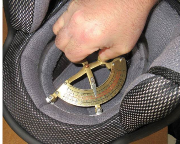
Figure 10. Measuring Discrete Size With Handheld Scissor Tool
