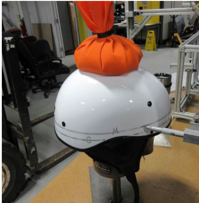
Figure 17. Helmet With Two Test Reference Lines
