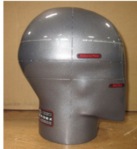
Figure 3. Test Reference Plane Location
