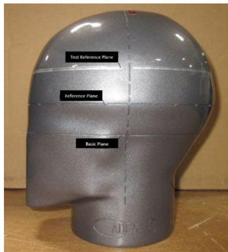
Figure B-1. Reference Headform with Test Reference Plane
