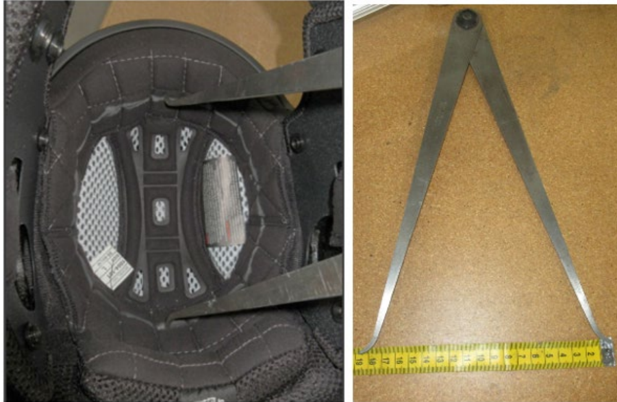
Figure 13. Internal Measurement (Uncompressed)
