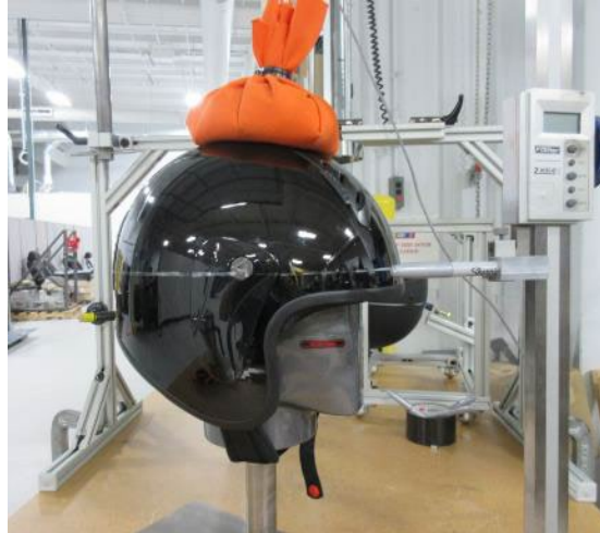
Figure 5. Test Reference Line Drawn on Helmet
