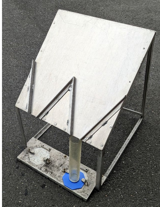
Figure 5. National Fire Protection Association 412 Splashboard with 1,000-mL Graduated Cylinder
