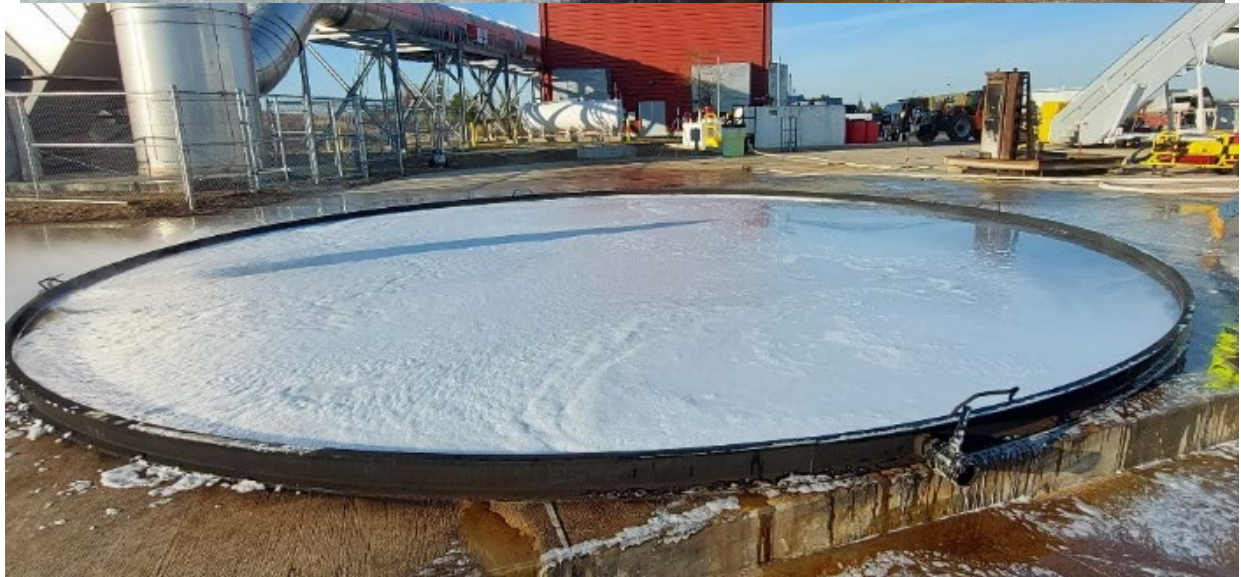
Figure 8. Foam Blanket After Standard (Top) and Foam Tube (Bottom) Discharges
