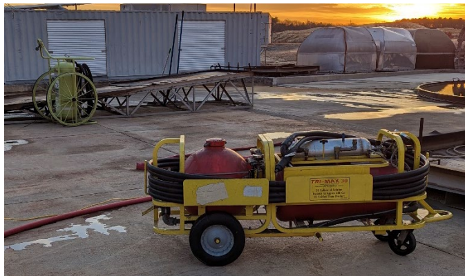
Figure 4. Novec 1230 Flightline Extinguisher (Rear Left) and TriMax Extinguishing System (Front Right)
