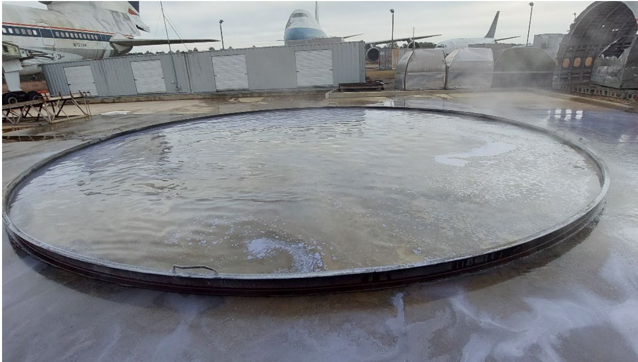
Figure 10. Pan Immediately After Extinguishment Using Dry Chemical Discharge
