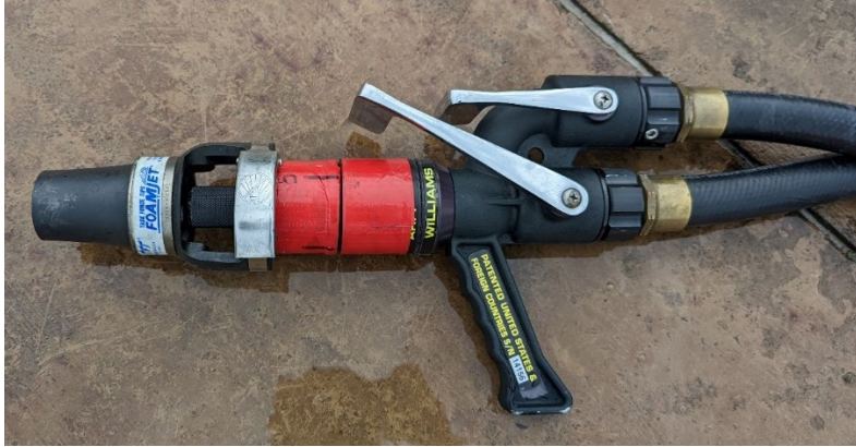
Figure 3. Williams Dual Agent Nozzle with Foam Tube Installed
