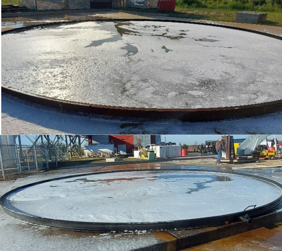
Figure 7. Chemguard C306 (Top) and Solberg AviGard (Bottom) Foam Blanket After Standard Discharge
