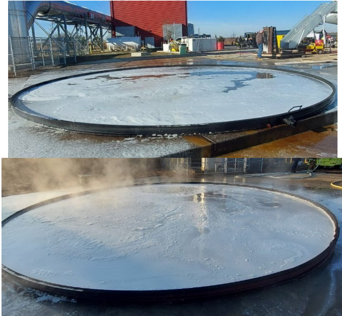
Figure 9. Foam Blanket After Standard (Top) and CAFS (Bottom) Discharges
