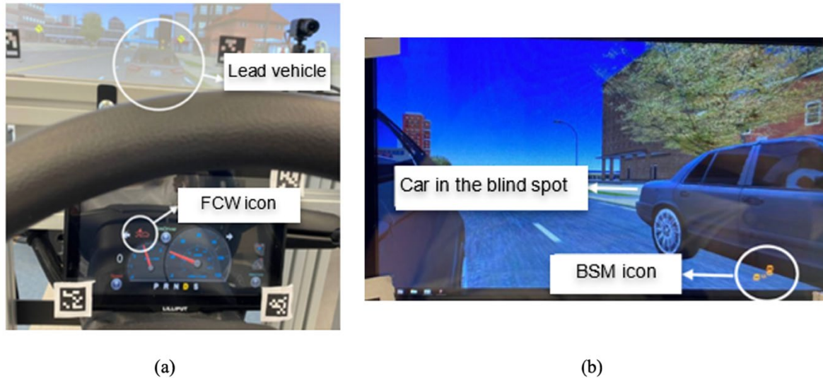
Figure 4. ADAS features in the driving simulation study: (a) FCW icon, (b) BSM icon.
