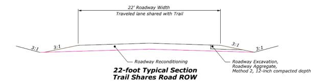
Figure 34 Road Typical Cross-Sections
