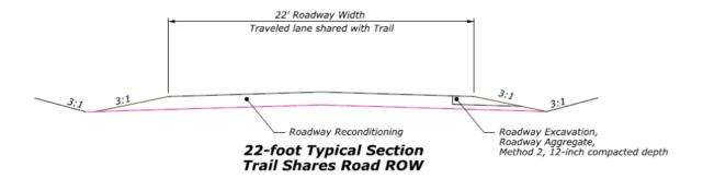
Figure ES- 3 Road Typical Cross Section
