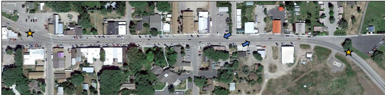
Figure 9. Location of data collection devices on Main St. (Notes: The stars indicate approximate locations of MetroCount traffic tube locations; the arrows designate approximate locations of CountCam2 traffic cameras pointing in the same direction of the camera orientation.)
