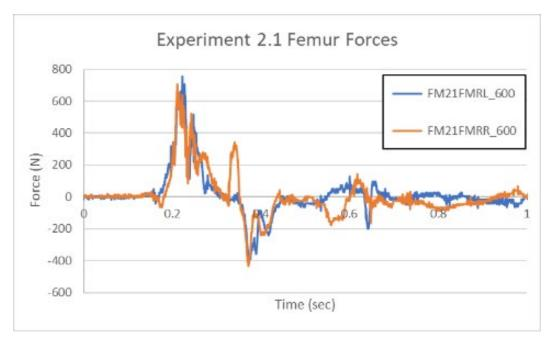
Figure 84. Occupant Protection Experiment 2.1 Femur Force Data
