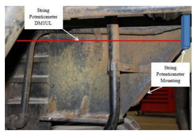
Figure 10. CEM Locomotive Underframe String Potentiometers
