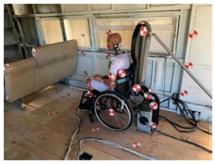
Figure 118. Post Impact Unrestrained Quantum Backboard
