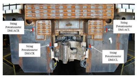
Figure 8. CEM Locomotive Coupler and Anti-Climber String Potentiometers
