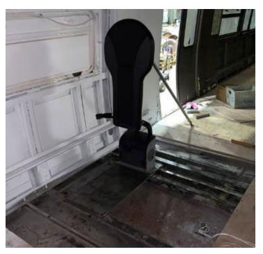
Figure 36. Quantum Backboard Restraint Device
