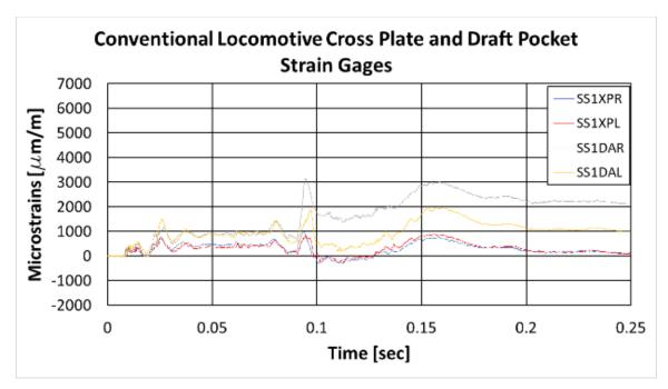
Figure 62. Conventional Locomotive Cross Plate and Draft Pocket Strain Results
