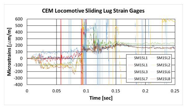
Figure 49. CEM Locomotive Sliding Lug Strain Results
