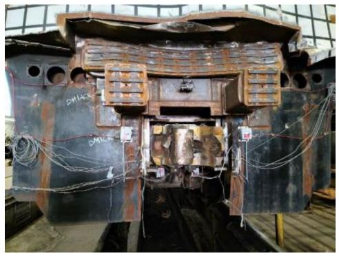
Figure 95. Crushed Upper DAC and Partially Crushed Lower DAC Tubes
