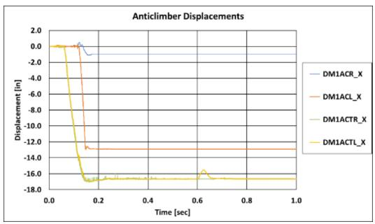
Figure 46. Anti-climber Displacements
