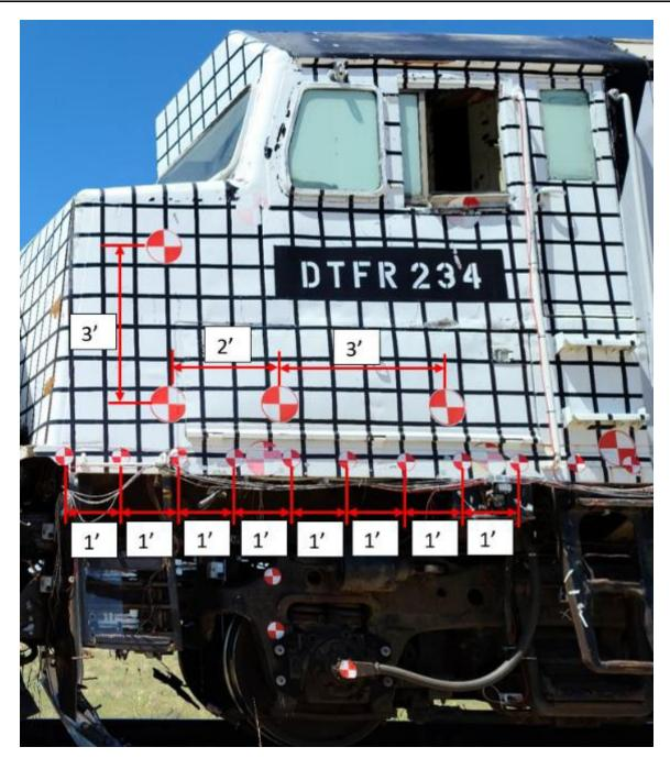
Figure A1. Target Spacing for CEM Locomotive
