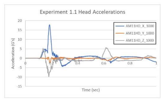
Figure 72. Occupant Protection Experiment 1.1 Head Acceleration Data
