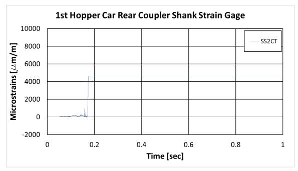
Figure 65. First Hopper Car Rear Coupler Shank Strain Results
