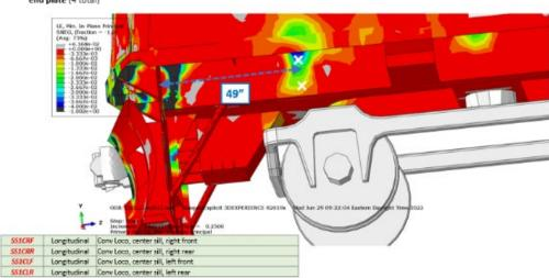
Center Sill: Two gages on each side of main I-beam webs - 2" above bottom flange and 2" below top flange, both 49" from front end plate (4 total)
