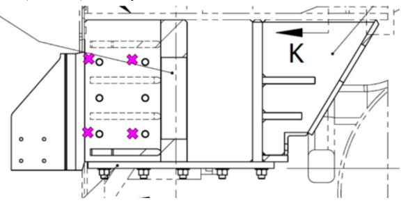
Figure 14. Strain Gage Locations on CEM Locomotive Sliding Lug
