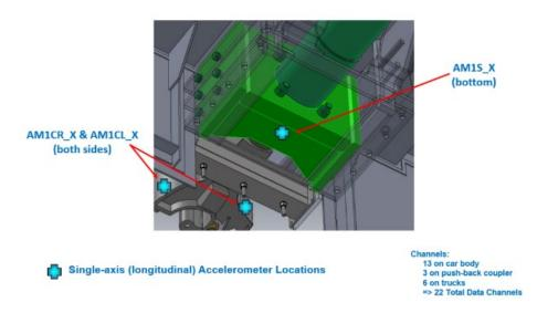
Figure 5. Locations of Accelerometers on CEM Locomotive Sliding Lug and Pushback Coupler
