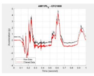
Figure B121. AM11PL\_Z Accelerometer Data
