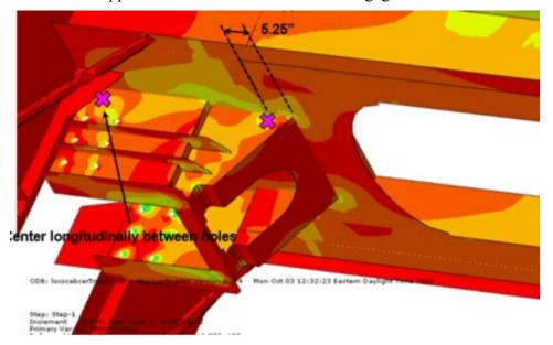
Figure 16. Strain Gage Locations on CEM Locomotive Draft Pocket
