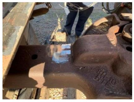
Figure 25. Strain Gage Location on the First M1 Passenger Car Lead Coupler
