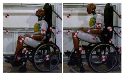
Figure 69. Occupant Protection Experiment 1.1 Impact Movement
