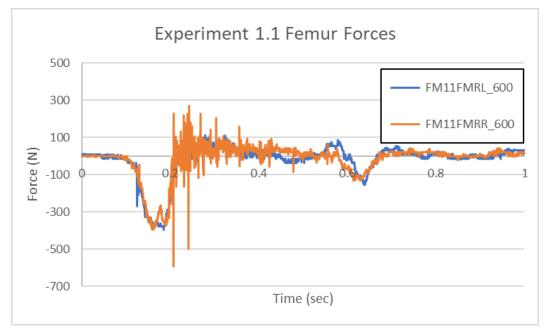
Figure 83. Occupant Protection Experiment 1.1 Femur Force Data
