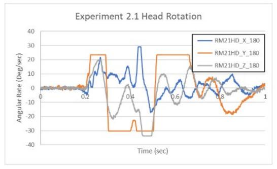
Figure 81. Occupant Protection Experiment 2.1 Head Rotation Data
