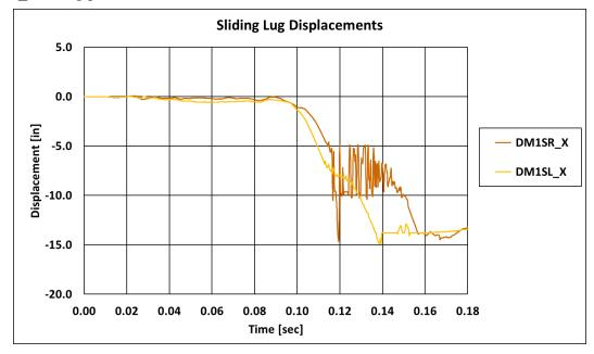
**Figure 47. Sliding Lug Displacements**
