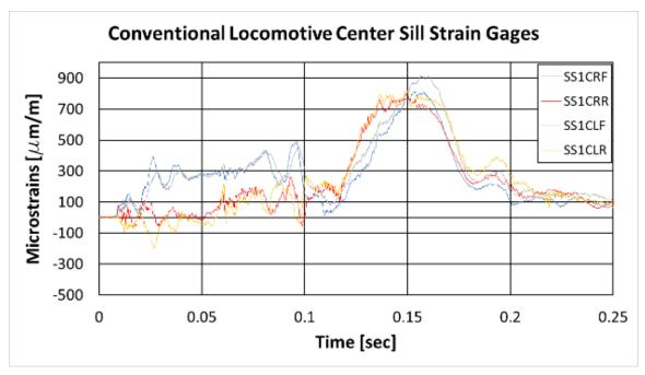
Figure 61. Conventional Locomotive Center Sill Strain Results
