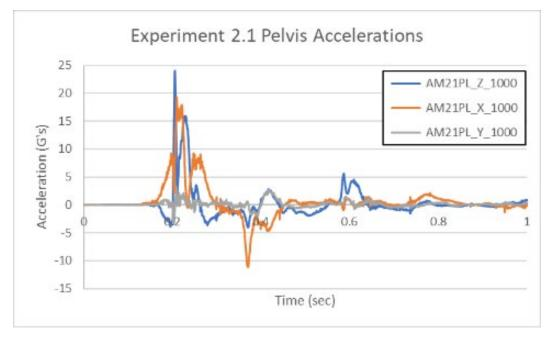
Figure 79. Occupant Protection Experiment 2.1 Pelvis Acceleration Data
