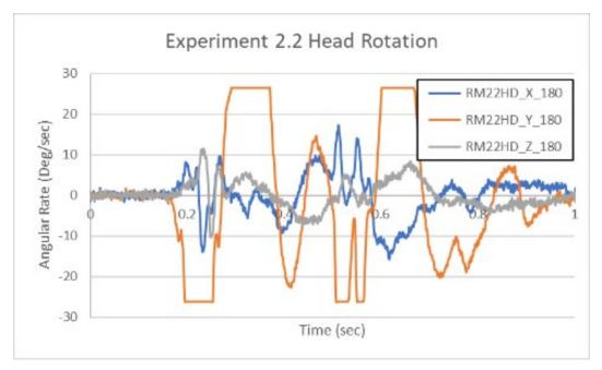
Figure 82. Occupant Protection Experiment 2.2 Head Rotation Data
