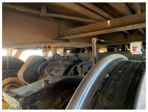
Figure 22. First M1 Passenger Car Lead Truck to Bolster String Potentiometers
