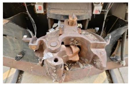
Figure 100. Conventional Locomotive Coupler Head – After Impact
