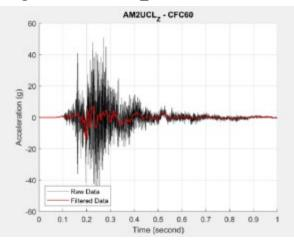
Figure B9. AM2UCL\_Z Accelerometer Data
