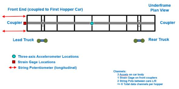
Figure 35. Second Hopper Car Instrumentation
