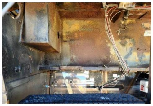
Figure 107. Curved Center Sill in Front End of CEM Locomotive
