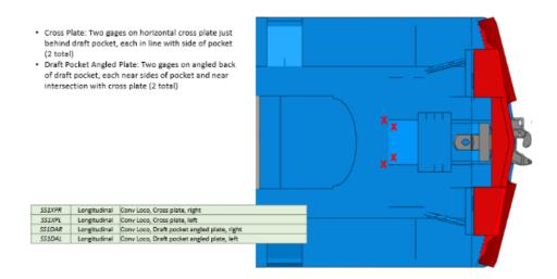
Figure 32. Strain Gages on the Cross-plate and the Draft Gear Pocket Back Plate
