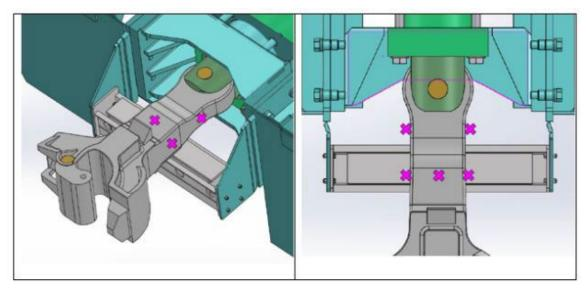
Figure 13. Strain Gage Locations on CEM Locomotive Coupler Shank
