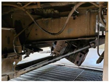
Figure 113. Yoke from the Front Coupler on Car 8332
