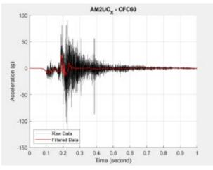
Figure B5. AM2UC\_X Accelerometer Data
