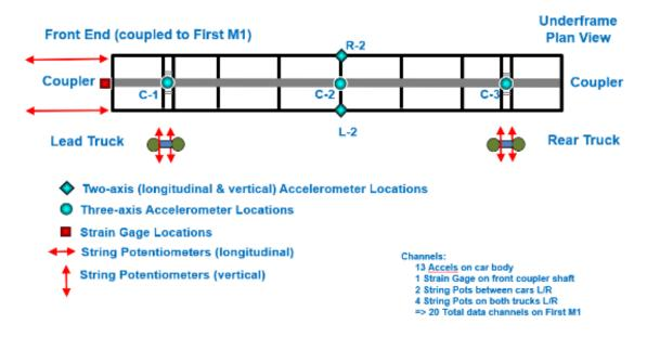
Figure 26. Second M1 Car Instrumentation
