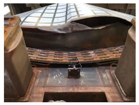
Figure 101. CEM Locomotive – Deformed Nose
