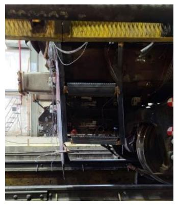
Figure 102. CEM Locomotive – Bent Front Plate
