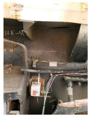
Figure 111. Buckled Floor Structure and Deformed Front Plate, Left Side
