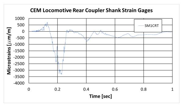
Figure 54. CEM Locomotive Rear Coupler Shank Strain Results
