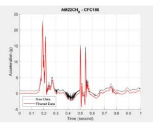
Figure B98. AM22CH\_X-CFC180 Accelerometer Data
