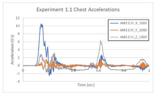
Figure 75. Occupant Protection Experiment 1.1 Chest Acceleration Data
