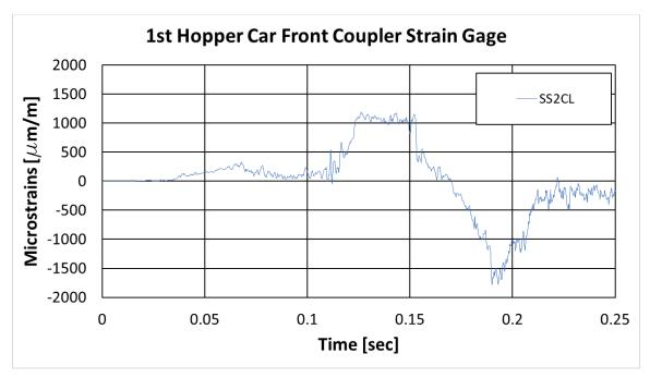
Figure 64. First Hopper Car Front Coupler Shank Strain Results
