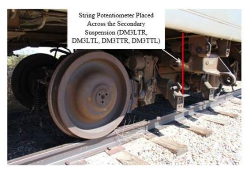
Figure 27. Second M1 Passenger Car Truck Secondary Suspension String Potentiometer
