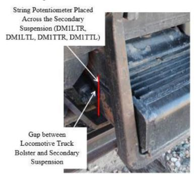
Figure 7. CEM Locomotive Truck Secondary Suspension String Potentiometer Location
