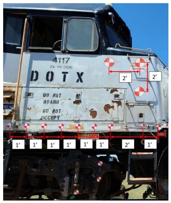
Figure A2. Target Spacing for Conventional Locomotive
