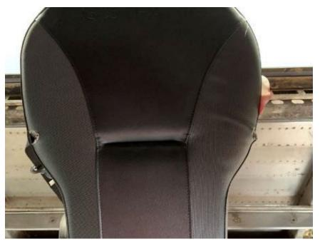
Figure 120. Holes in the Left and Right Side of the Full Quantum System Backboard
