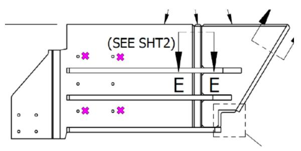
Figure 15. Strain Gage Locations on CEM Locomotive Draft Pocket
