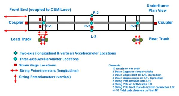
Figure 19. First M1 Passenger Car Instrumentation
