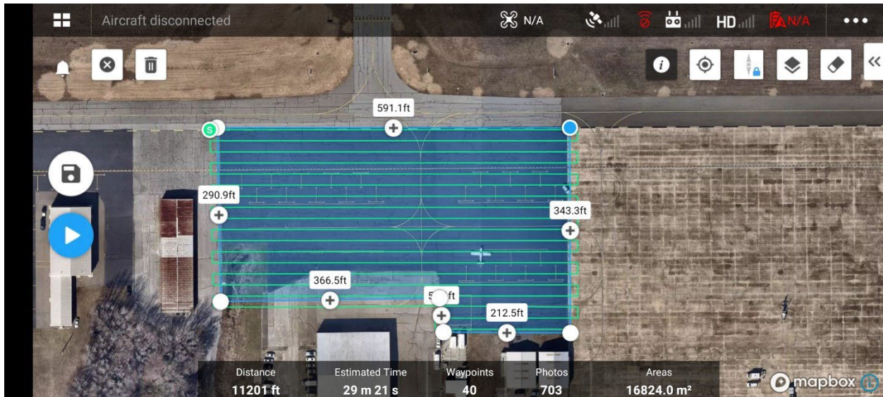
Figure B-6. Flight Plan for Stereo Thermal Data Collection with Mavic 2 Enterprise Advanced Over Apron 30
