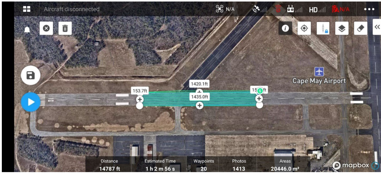
Figure B-5. Flight Plan for Stereo Thermal Data Collection with Mavic 2 Enterprise Advanced Over Part of Runway 10/28
