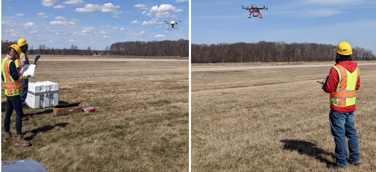
Figure 21. High-Resolution sUAS Data Collection with mdMapper1000+ and Bergen Hexacopter sUAS Platforms
