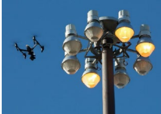
Figure A-7. Image of sUAS for High-Mast Lighting Pole Inspection by NJDOT (FHWA, 2018b)
