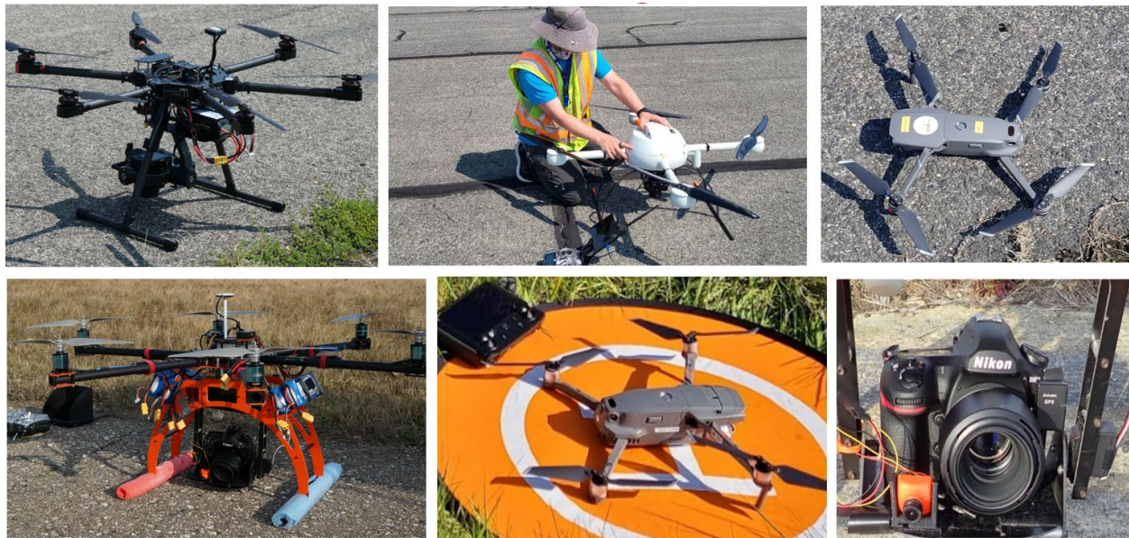
Figure 93. Examples of sUAS Platforms and Sensors Deployed (Clockwise, from top left: Tarot X6 with Nikon D850, mdMapper1000+, Mavic 2 Pro, Nikon D850 camera, M2EA [on top of orange landing pad], Bergen Hexacopter with Nikon D850 ready for deployment)
