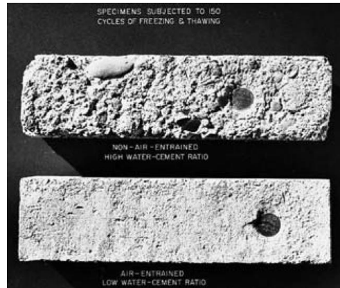
Figure 7. Air-entrained concrete (bottom bar) is highly resistant to repeated freeze-thaw cycles (Kosmatka et al. 2011)
