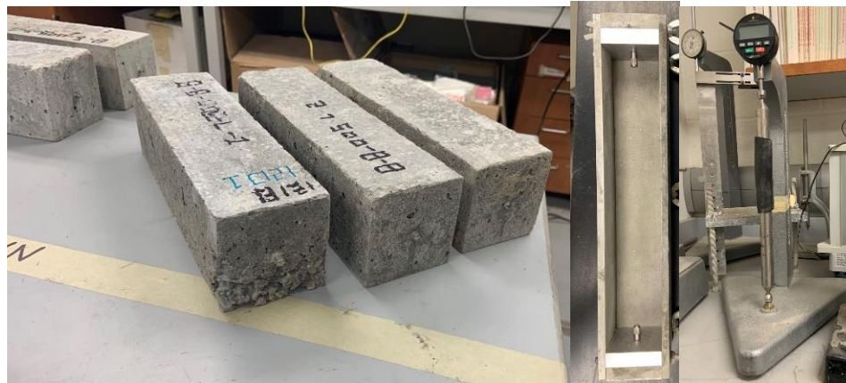
Figure 18. 3-in. by 3-in. by 11.25-in. prism drying shrinkage specimen, drying shrinkage molds, and measurement apparatus
