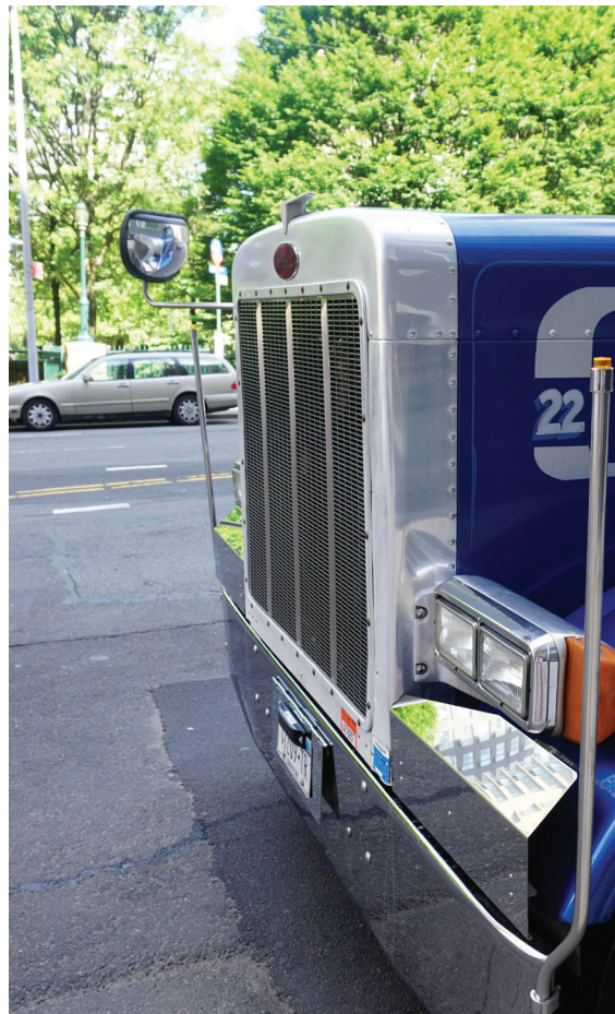
Truck-mounted crossover mirror
