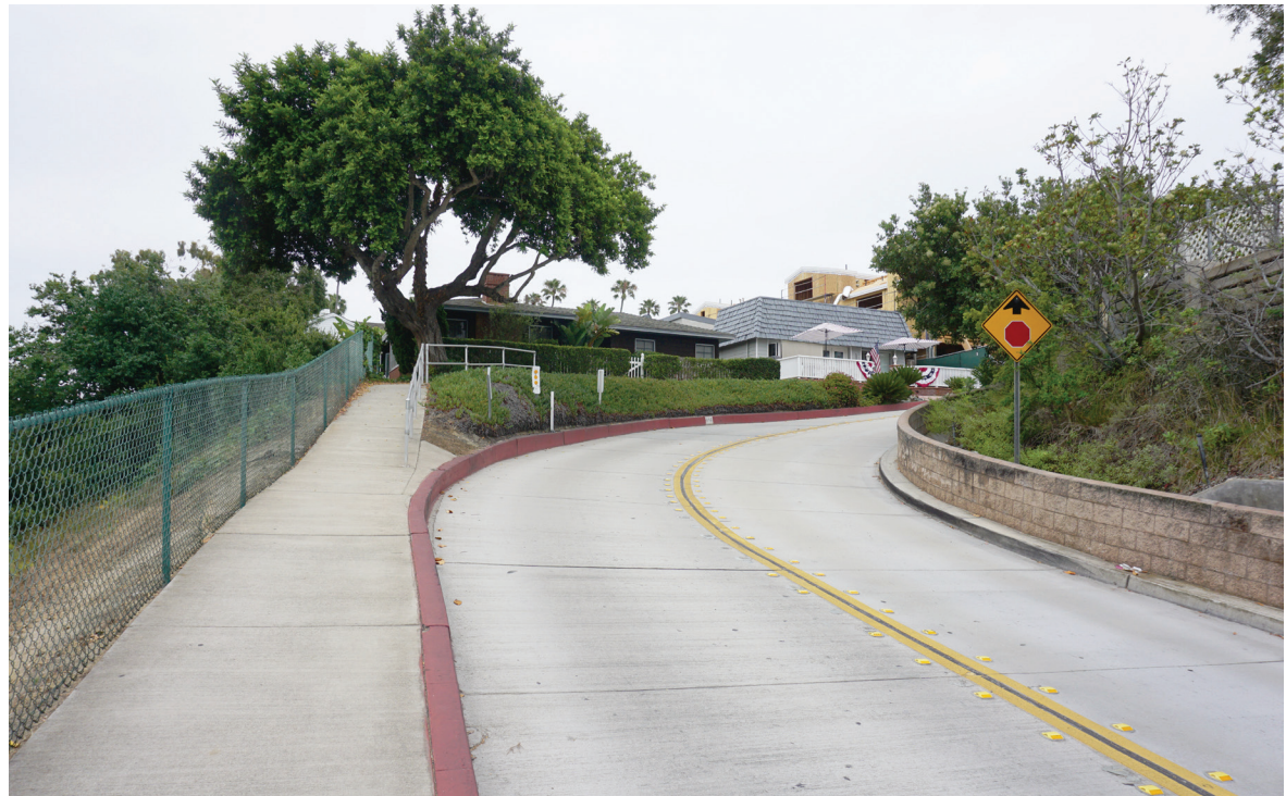
Painted curb to indicate parking prohibited
