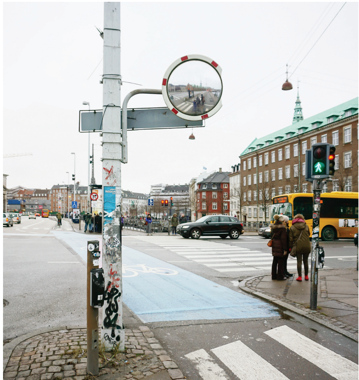
Convex safety mirror mounted to lightpost
