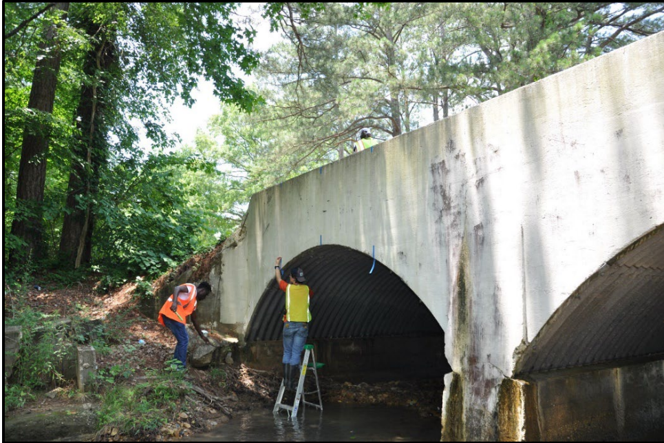
Figure 5.20. Location of instrumentation points at the Bain's Gap Road culvert.
