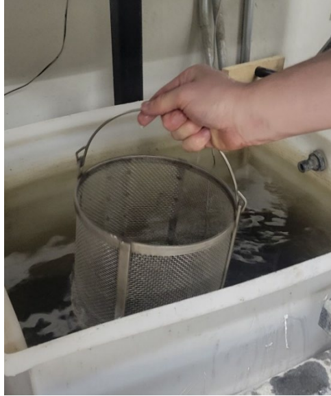
Figure 4.2 Aggregate Submersion in Water Bath
