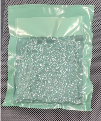
Figure 4.9 Vacuum Sealed CoreLok Bag with Coarse Aggregate
