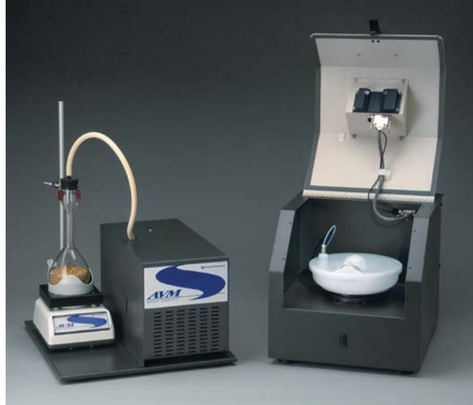
Figure 2.1 SSDetect System used to identify the SSD condition of Fine Aggregates (For Construction Pros.com, 2022)
