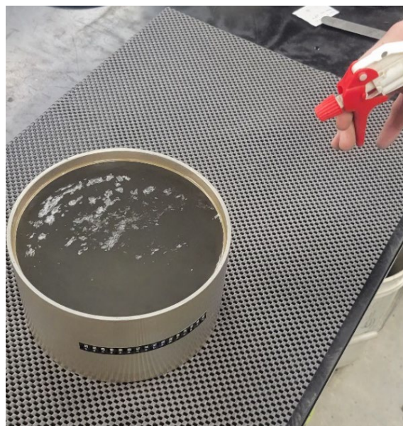
Figure 4.5 Spraying Isopropyl Alcohol on the Water Surface of the Volumeter
