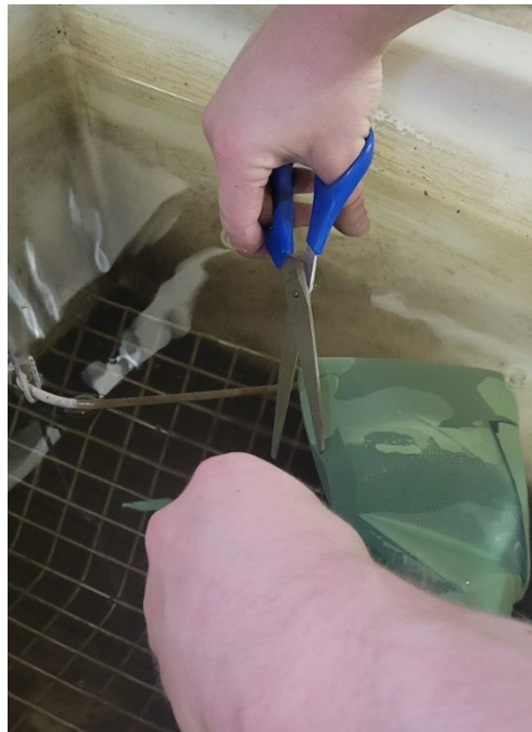
Figure 4.10 Cutting Vacuum Sealed Bag Under Water
