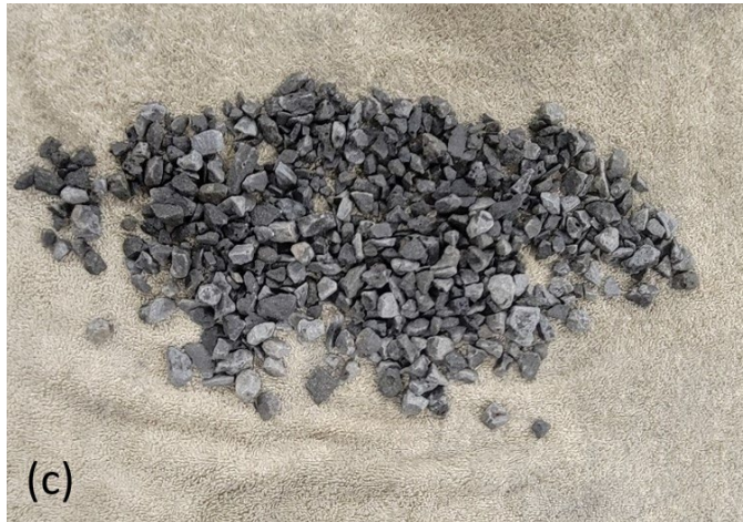
Figure 4.1 Aggregate Appearance at Various Stages of Drying. (a) “Shiny” Aggregate on wet side of SSD, (b) Aggregate at SSD Condition, and (c) Aggregate on dry side of SSD
