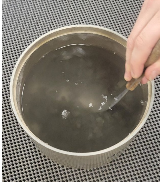
Figure 4.4 Stirring the Aggregate Sample in a Cross Pattern
