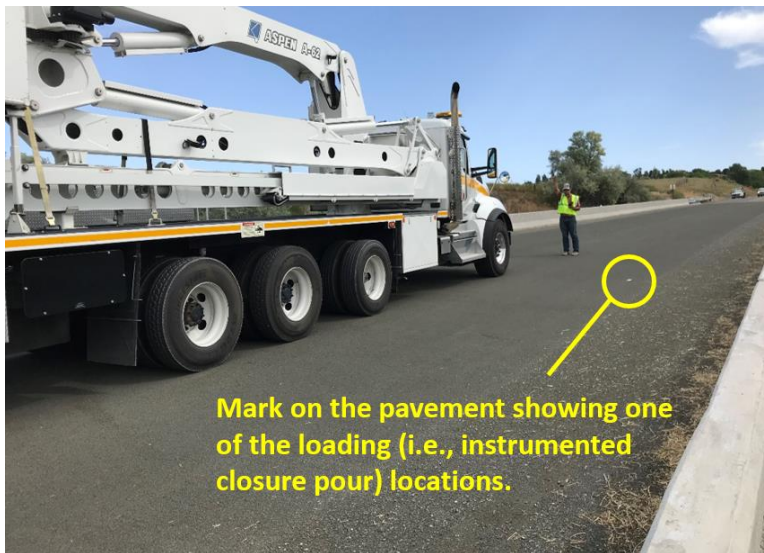
Figure 2-8 UBIT loading position for Test 3
