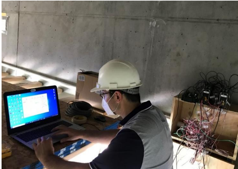
Figure 2-7 Data acquisition system under the bridge
