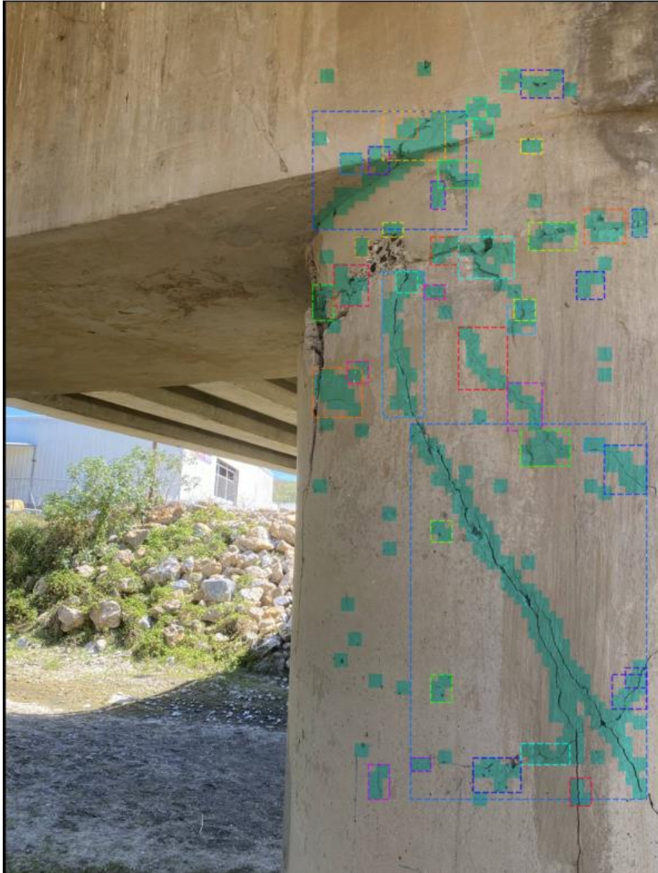
Figure 6.26 – Computer Vision Analysis Results for Real Earthquake Caused Damaged RC Bridge Column
