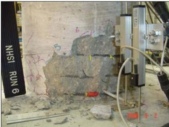
Damage State IV (4.20%)
