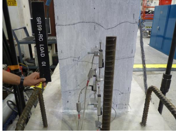
Damage State I (0.5% Drift)
