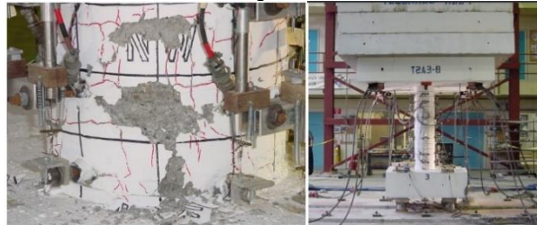
Damage State III (7.62%, 7.63%)
