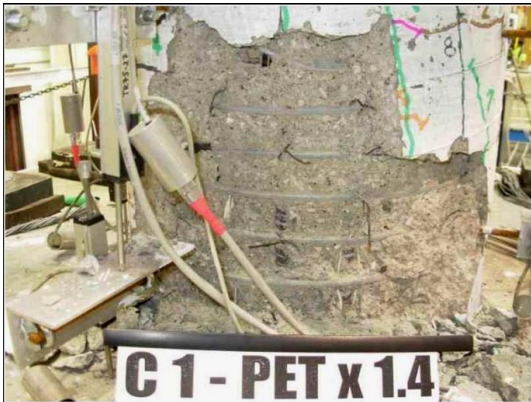
Damage State IV (8.33%)
