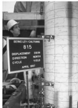
Damage State II (1.82%)
