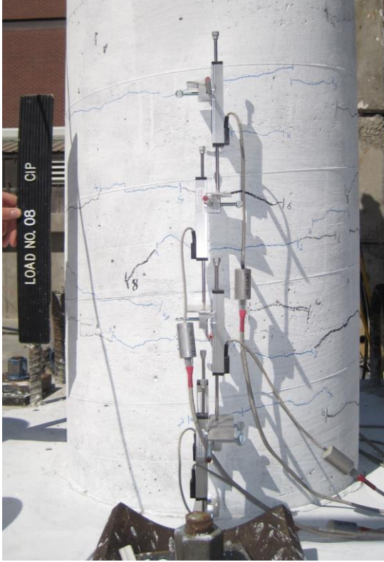
Cast-in-Place Column by Haber et al. (2013) Photo at Drift Ratio: 0.5% Column Height = 108 in. Diameter = 24 in.
