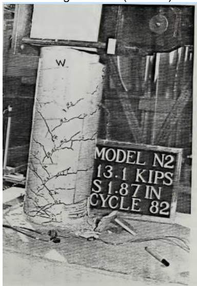
Damage State IV (5.97%)
