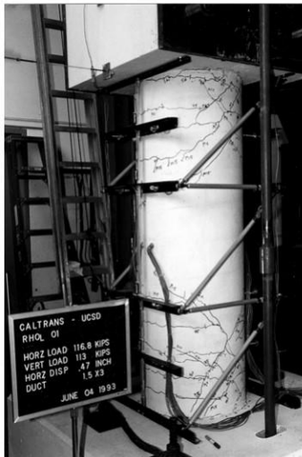
Damage State II (0.52%)
