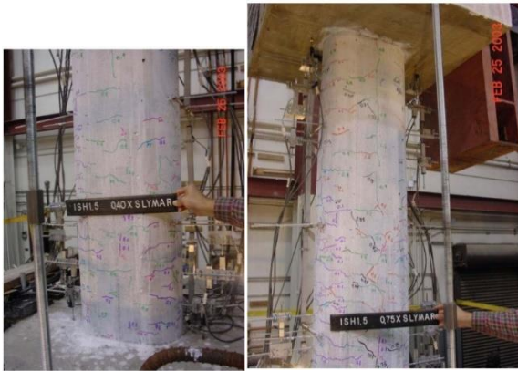
Damage State II (1.3%, 1.87%)
