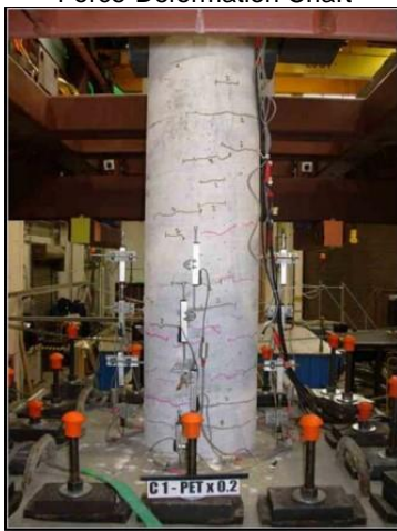
Damage State II (0.91%)
