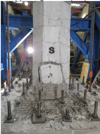
(e) Damage State 5 (DS5)
