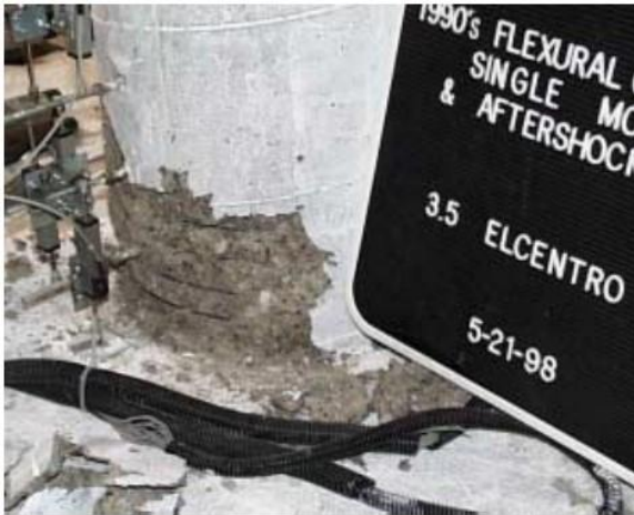
Damage State IV (6.94%)
