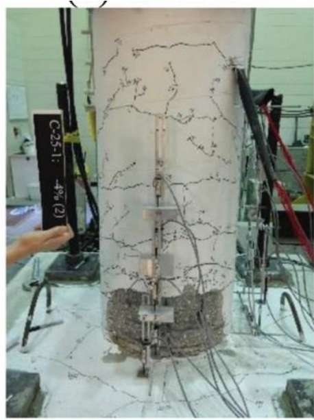
Damage State IV (4%)
