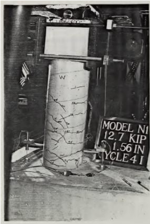
Damage State II (5.15%)
