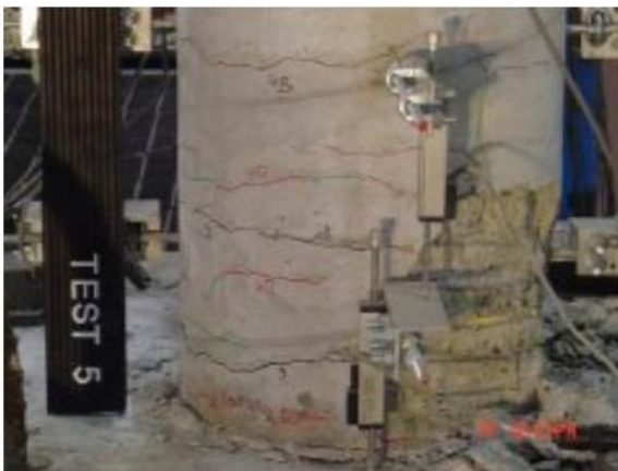
Damage State IV (4.4%)
