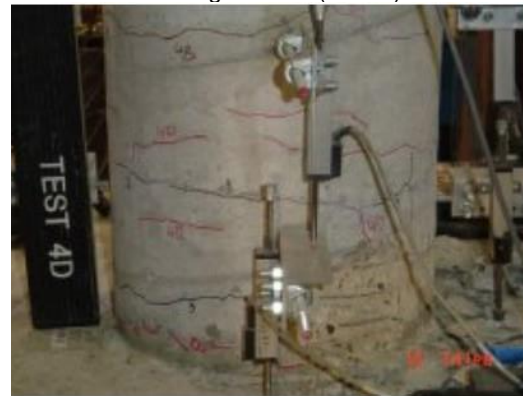
Damage State III (2.71%)
