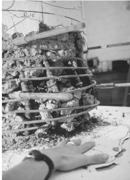
Damage State VI (7.42%)
