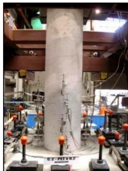
Damage State II (0.567%)
