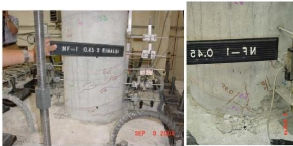
Damage State II (4.44%, 4.44%)
