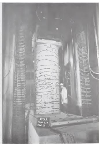
Damage State II (1.5%)
