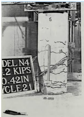
Damage State II (1.42%)
