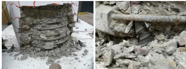
Damage State V (9.73%) & VI (10.62%)
