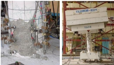
Damage State IV (14.1%, 14.1%)
