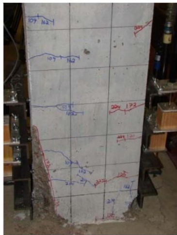
Damage State IV (3.43%)
