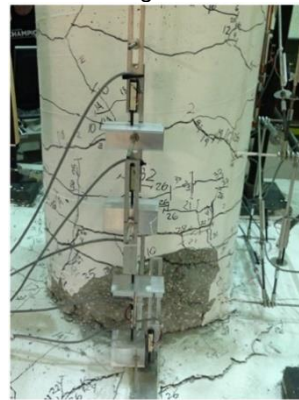
Damage State III (5%)
