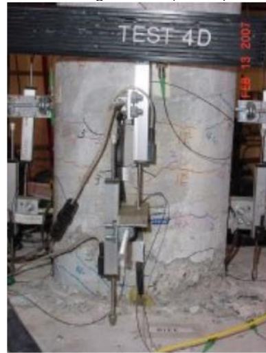
Damage State III (2.62%)
