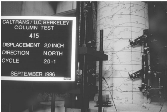
Damage State II (2.08%)
