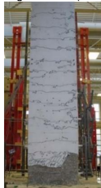
Damage State IV (2.89%)
