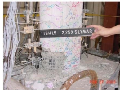
Damage State III (3.86%, 4.35%)
