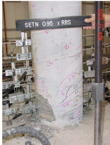
Damage State IV (5.65%, 8.02%)
