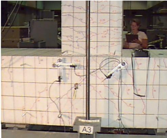
Damage State II (0.9%)
