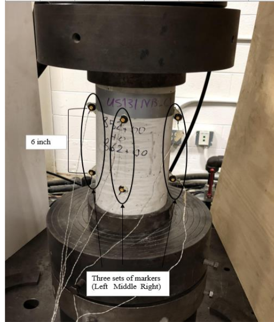
Figure 49 Elastic modulus and compressive strength test setup
