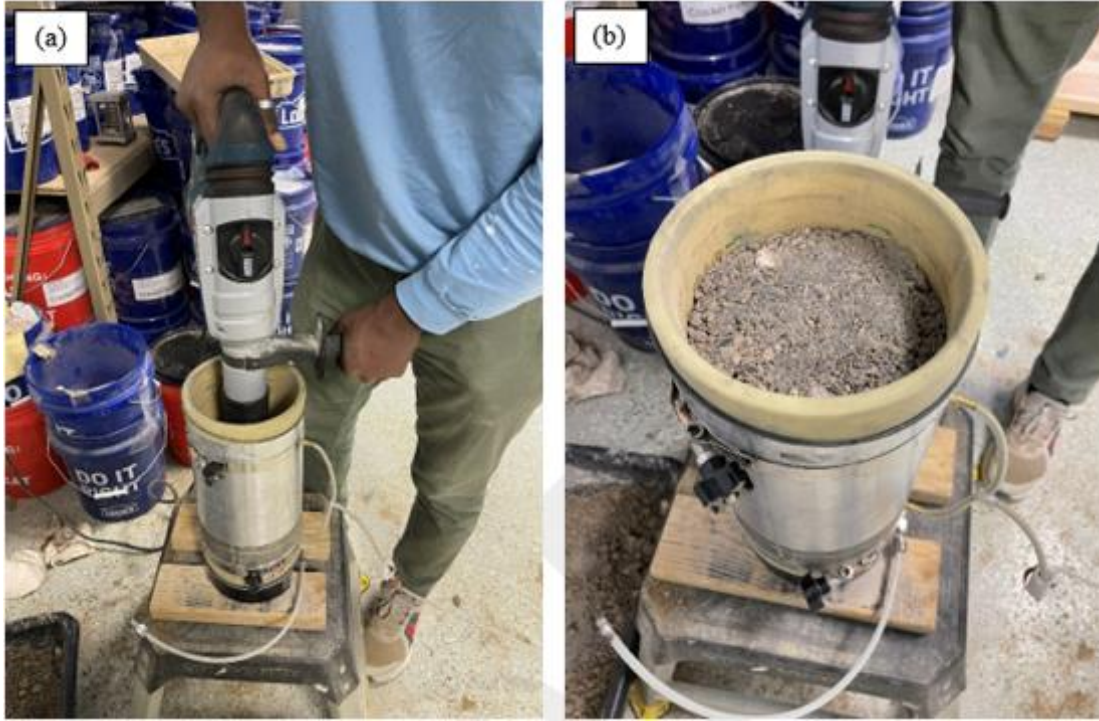
Figure 72 (a) Compaction with vibrating hammer and (b) compacted specimen
