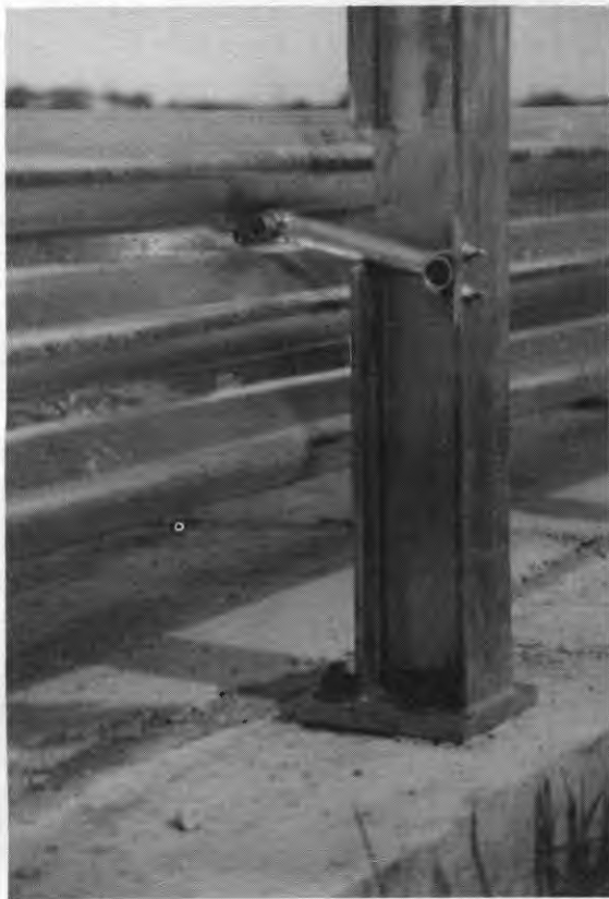
FIGURE 74. SELF-RESTORING THRU-TRUSS RETROFIT TEST INSTALLATION
