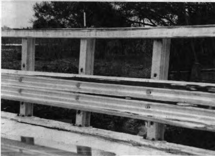
FIGURE 66. TEST TTR-1 BARRIER DAMAGE
