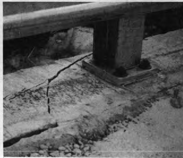
FIGURE 66. TEST TTR-1 BARRIER DAMAGE
