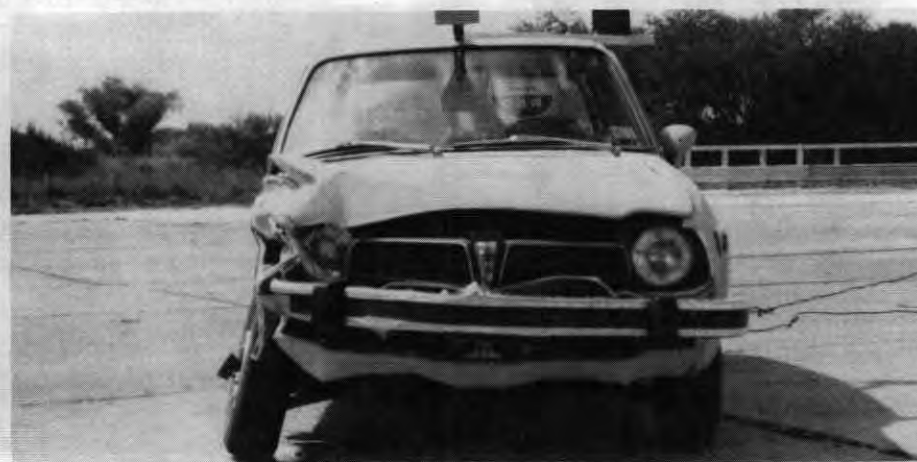
FIGURE 100. BARRIER AND VEHICLE DAMAGE, TEST TTR-10
