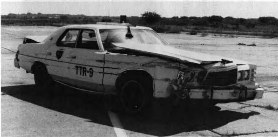
FIGURE 97. BARRIER AND VEHICLE DAMAGE, TEST TTR-9
