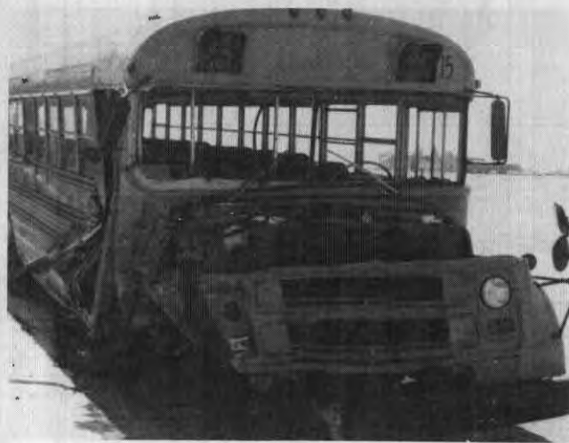
FIGURE 85. BARRIER AND VEHICLE DAMAGE, TEST TTR-5
