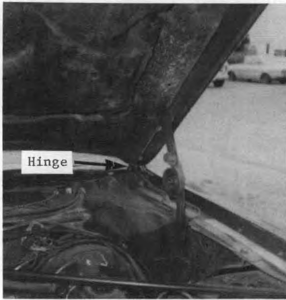
(e) 1980 Chrysler Newport hinge detail
