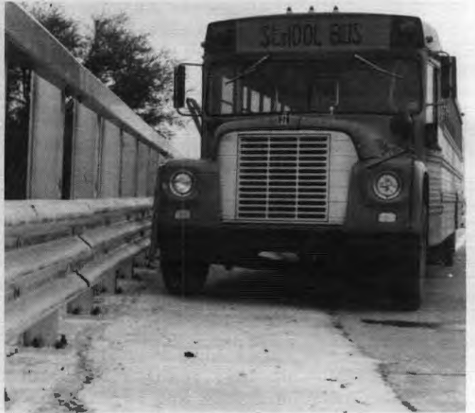
FIGURE 63. THRU-TRUSS RETROFIT TEST INSTALLATION
