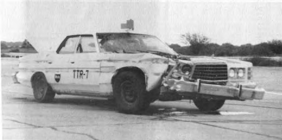
FIGURE 91. BARRIER AND VEHICLE DAMAGE, TEST TTR-7
