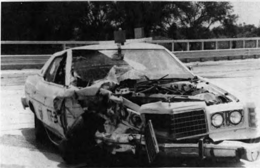
FIGURE 94. BARRIER AND VEHICLE DAMAGE, TEST TTR-8
