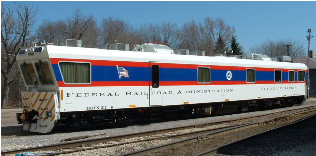
Figure 1. FRA DOTX 217 Track Geometry Car (FRA, 2019)
