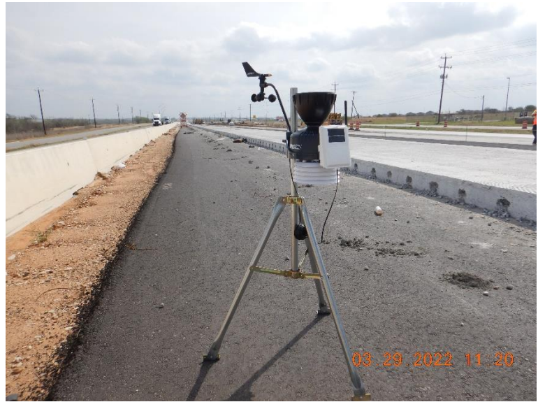
Figure 5.2 Davis Weather Station installed in field test site
