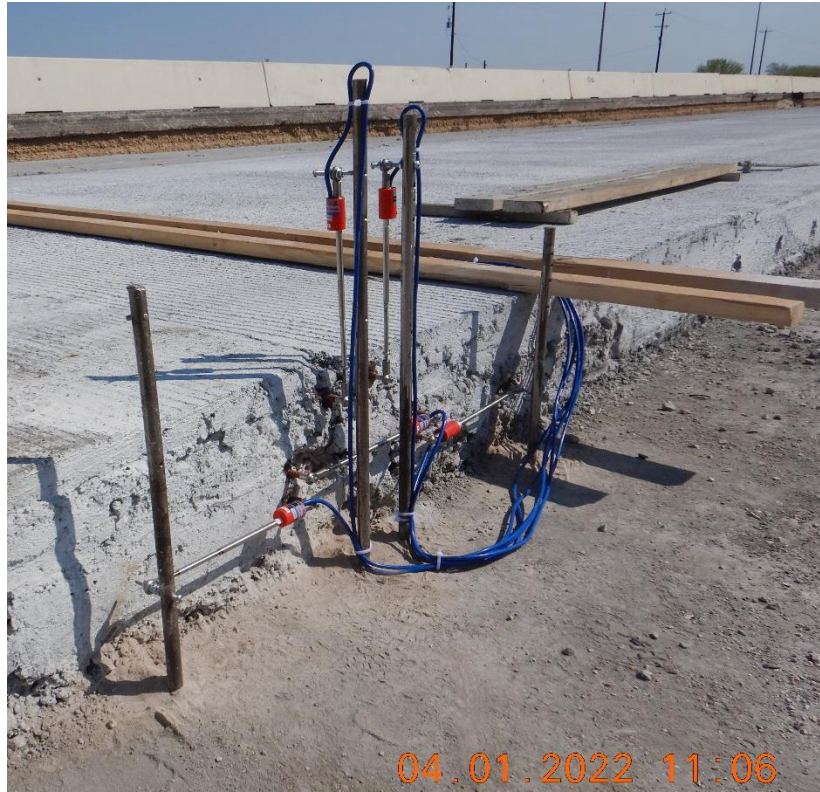
Figure 5.5 Typical Installation of Crackmeter in the field
