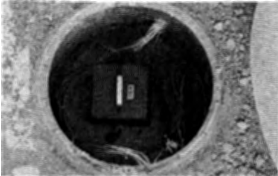
Figure 53.- Meloland overcrossing. View downward of FBA-3 accelerometer package anchored to small reinforced-concrete pad at bottom of ground vault.
