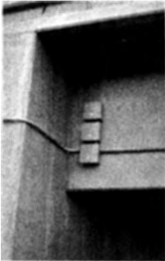
A , View eastward of three FBA-1 accelerometers in metal boxes anchored to deck near abutment 3.
