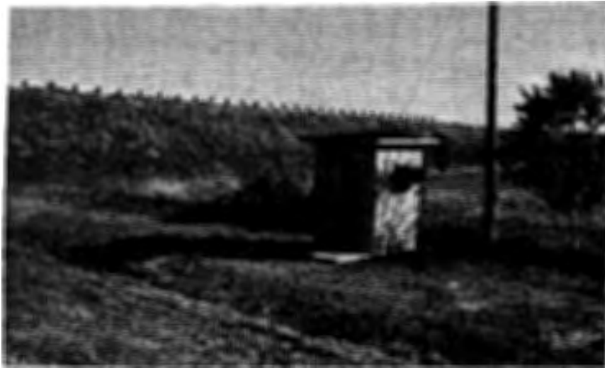
A , Shelter housing CR-1 recorder system; note air conditioner attached to side of shelter.
