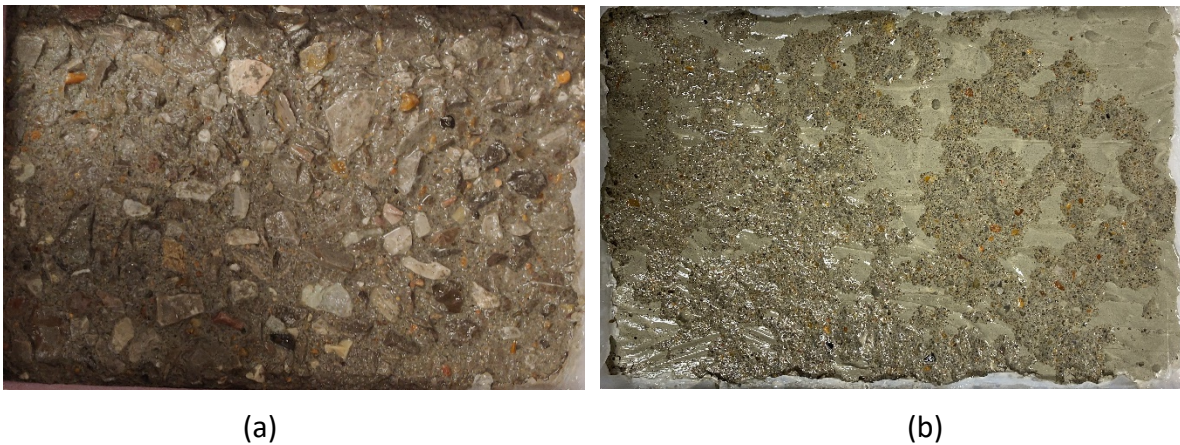
Figure 28. Photo. Degradation comparison after 20 cycles between two 0.5 w/cm concrete mixtures containing fly ash: (a) without air and (b) with air entrainment.
