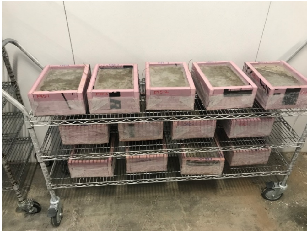
Figure 7. Photo. Salt-scaling slab specimen on wire cart.
