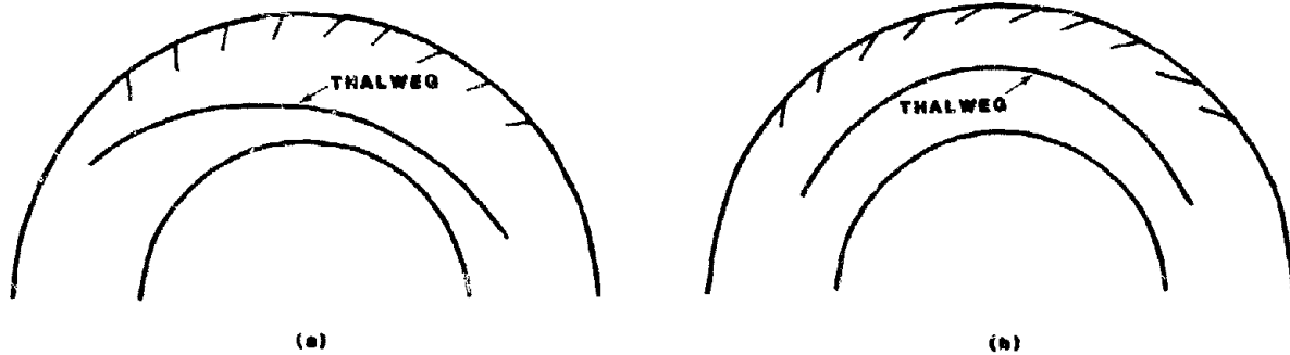
FIGURE 46. COMPARISON OF THALWEG POSITIONS PRODUCED BY SPURS ANGLED AT (A) 120 DEGREE, AND (B) 150 DEGREES.
