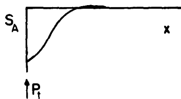
Fig. 6.3. Slope of pile caused by lateral load at groundline (Reese and Matlock, 1956).
