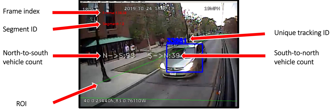
Figure 4.3: An example of a detected, tracked, and counted vehicle. The proposed system outputs bidirectional traffic counts. The segment ID indicates the current road segment occupied by the bus.
