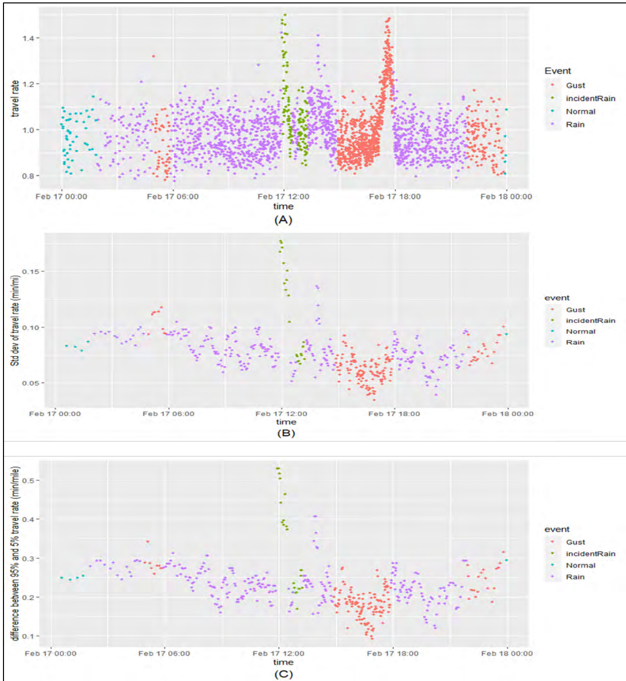
FIGURE D.6: (A): TRAVEL RATE VARIATION WITH TIME ON FEB 17, 2011. (B): VARIATION OF GROUP STANDARD DEVIATION (B) AND THE DIFFERENCE BETWEEN 95 TH AND 5 TH PERCENTILES (C) WITH TIME DURING THE SAME DAY.
