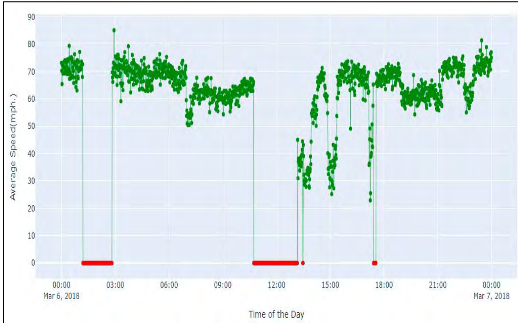
FIGURE 5.2: MISSING DATA OCCURRING AT REGULAR TIME INTERVALS FROM 01:11 AM TO 02:44 AM FOR SCHEDULED DETECTOR SYSTEM MAINTENANCE AND AT IRREGULAR TIME INTERVALS FROM 10:44 AM TO 13:10 PM ON 03/06/2018
