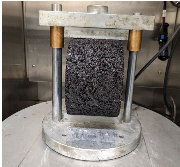
Figure 10. Photo. A specimen on the TSR fixture.
