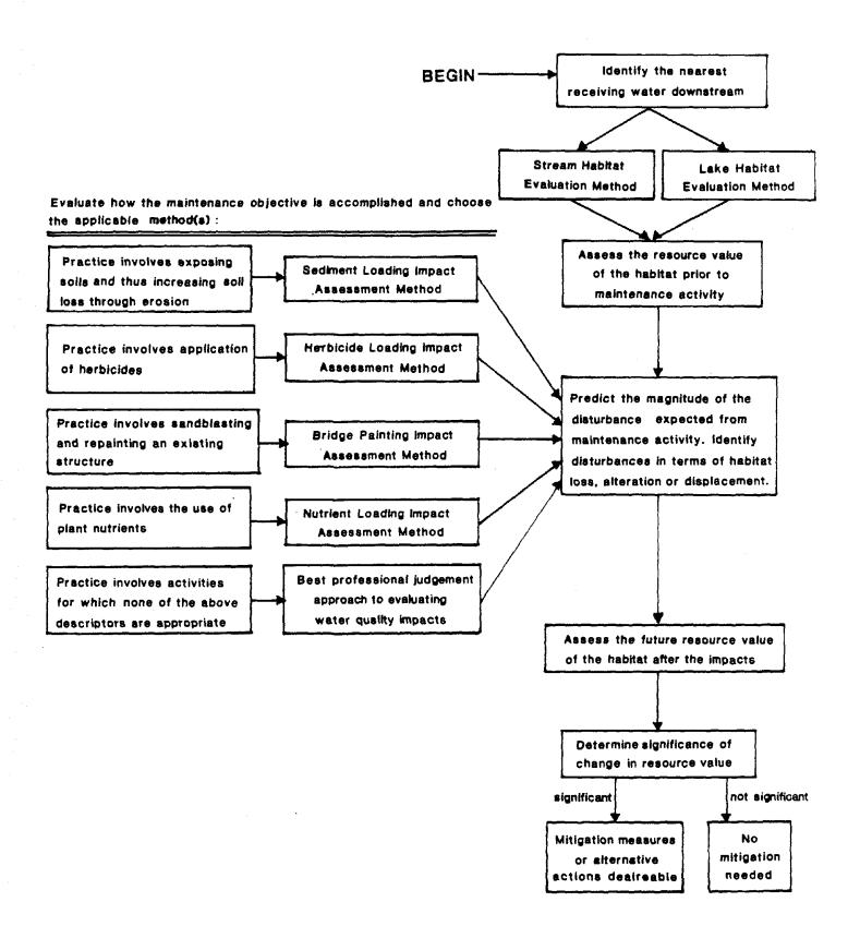
Figure 1. General impact assessment method for evaluating potential impacts to water quality from highway maintenance practices.
