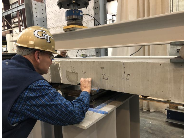
Figure 150. Photo. Researcher marking deepening cracks in the precast concrete panels at 20 kip load.
