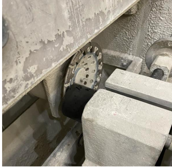
Figure 46. Photo. Grinding a 3 in. by 6 in. cylinder to ensure smooth testing surface.
