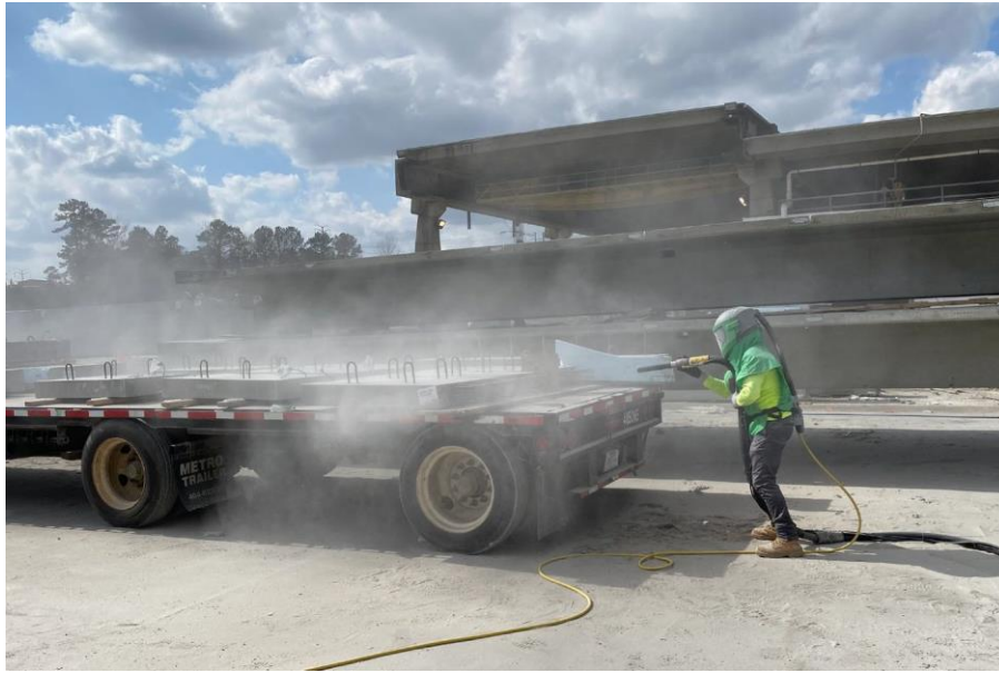
Figure 86. Photo. Sand blasting to create EA surface on specimens.
