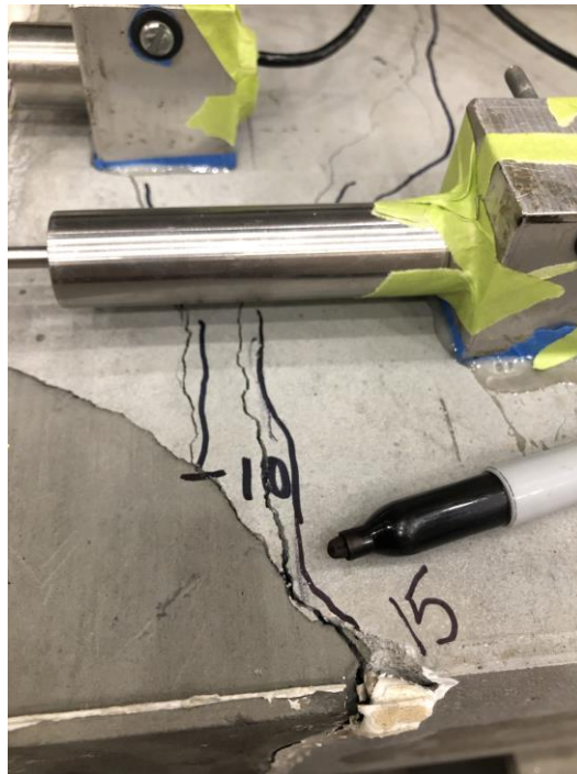
Figure 152. Photo. Cracks near UHPC joint propagating across the top of the specimen.
