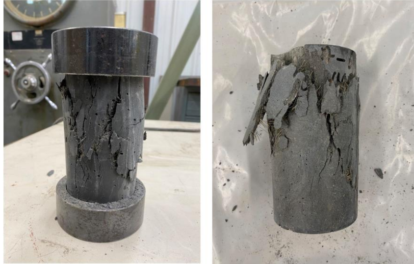
Figure 58. Photo. 3 in. by 6 in. cylinders after compression tests.
