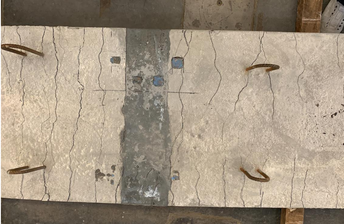
Figure 111. Photo. Specimen N-6-5.75-A tension side at failure.
