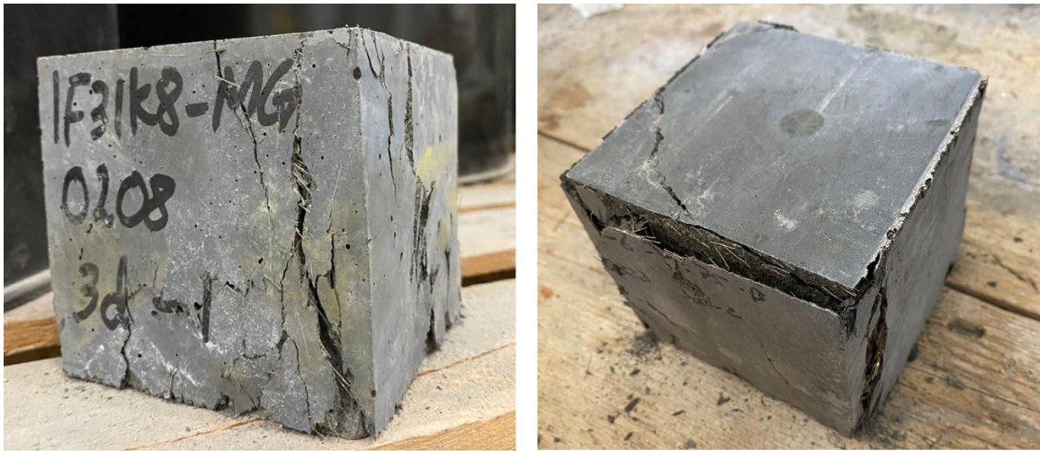
Figure 56. Photo. Failure mode of 100 mm UHPC cube specimens after compressive strength test.
