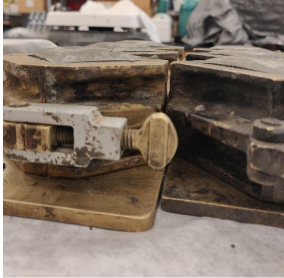
Figure 29. Photo. Mix 10MK showing expansion above the molds.
