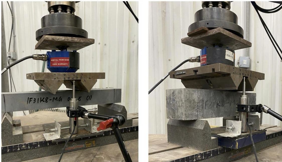
Figure 48. 2 in. by 2 in. by 17 in. beam (left) and 3 in. by 3 in. by 12 in. beam (right) during testing.
