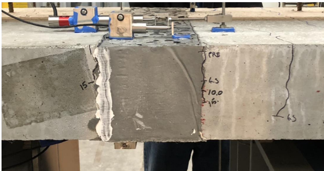
Figure 134. Photo. Cracks surrounding UHPC joint on north face at 15 kips.
