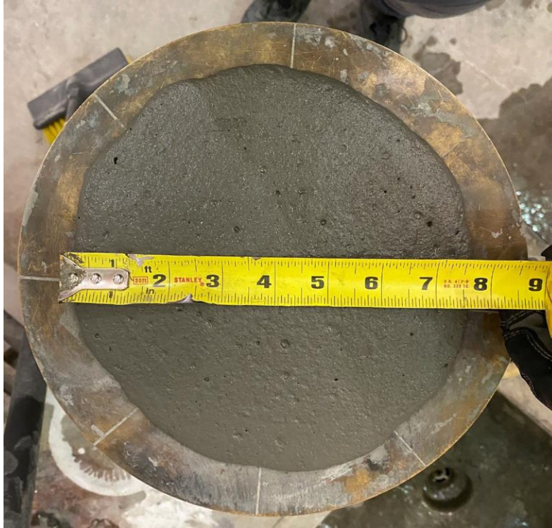
Figure 51. Photo. Flow diameter of 7-5/8 in. indicative of poor workability.
