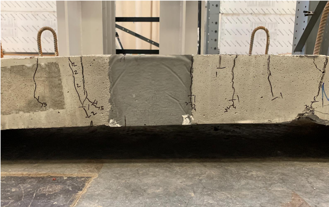
Figure 110. Photo. Specimen N-6-5.75-A showing concrete panel crushing.
