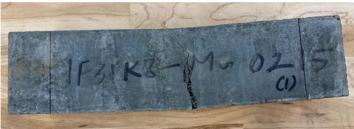
Figure 67. Photo. Major crack in the middle third of a 3 in. by 3 in. beam.
