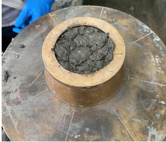
Figure 53. Photo. Indication of poor workability of a UHPC batch with 0.12 metakaolin-to- cement ratio.
