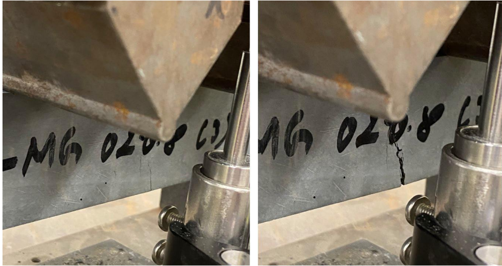
Figure 59. Photo. Formation of a major crack in a beam specimen during four-point bending test.
