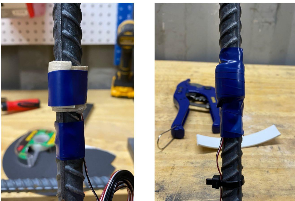
Figure 75. Photo. Foam tape and electrical tape used to protect the attached strain gauge.
