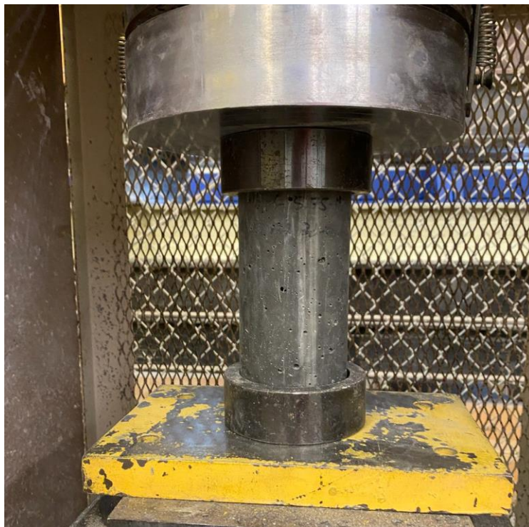
Figure 45. Photo. 3 in. by 6 in. UHPC cylinder ready for testing.
