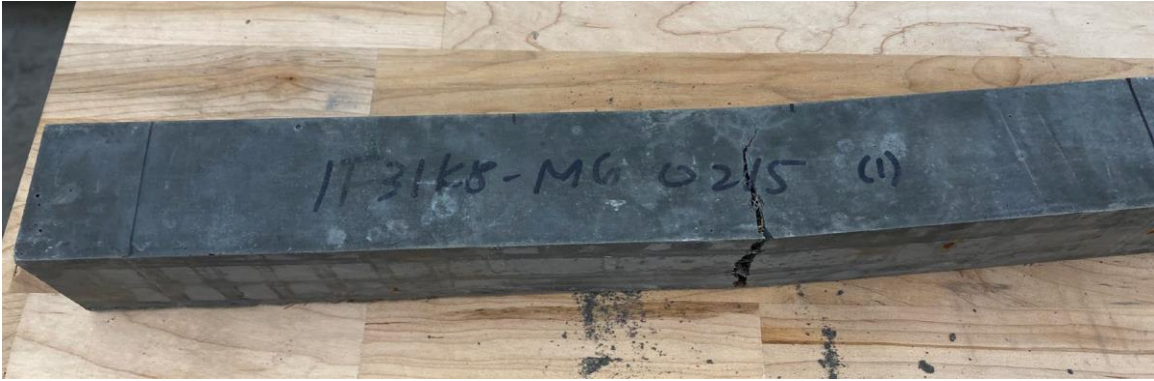
Figure 65. Photo. Major crack in the middle third of a 2 in. by 2 in. beam.
