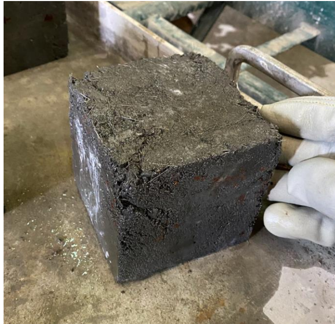
Figure 42. Photo. 100 mm cube specimen. The shape is distorted due to poor workability of UHPC.
