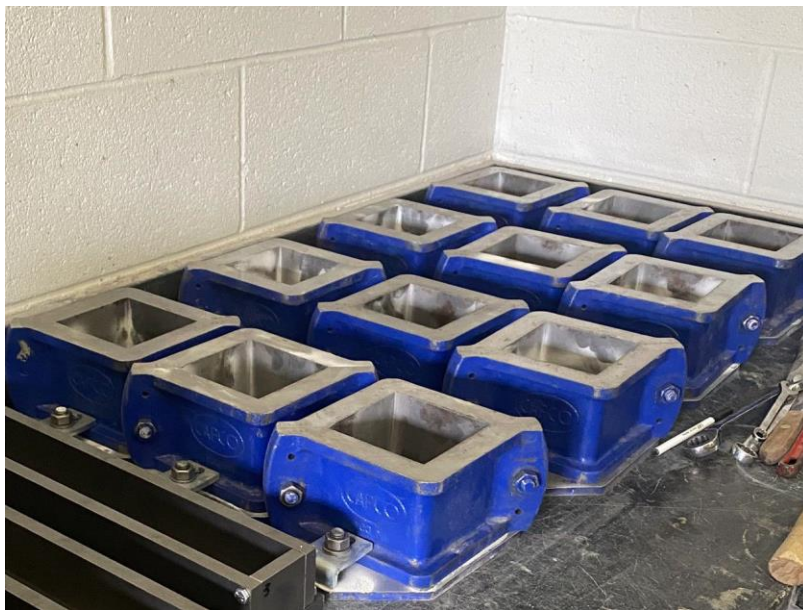
Figure 43. Photo. 100 mm cube molds used for casting UHPC.
