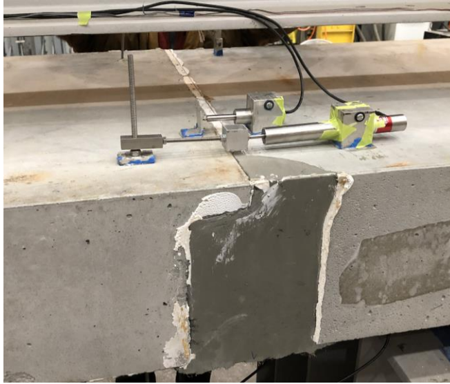
Figure 148. Photo. UHPC cast around damaged shear key.
