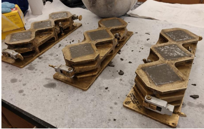
Figure 24. Photo. Mortar cube specimens being cast for compression testing.
