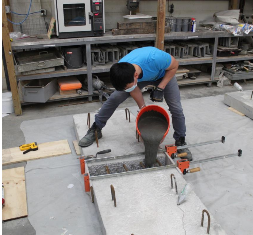
Figure 93. Photo. UHPC joint pour.
