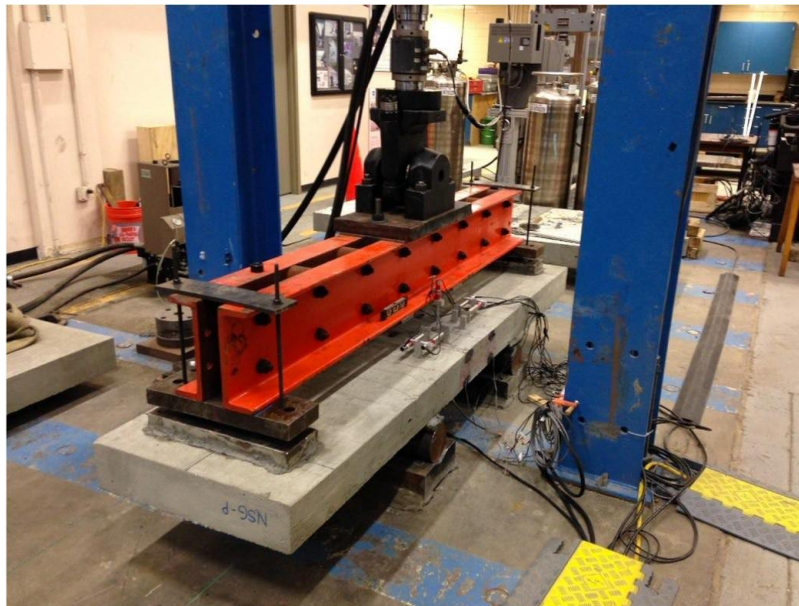
Figure 16. Photo. Deck panel specimen during loading. (40)
