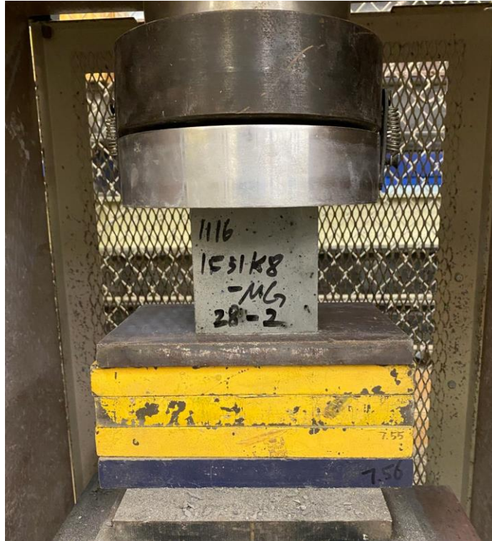
Figure 44. Photo. 100 mm UHPC cube specimen ready for testing.
