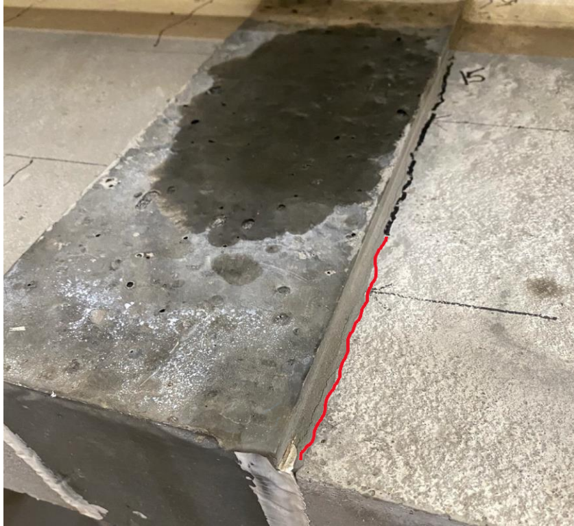
Figure 101. Photo. Propagation of interface crack at M_y .
