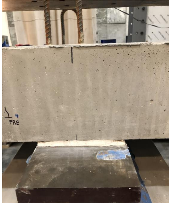
Figure 129. Photo. Closeup of ¼ in. gap filled with Hydrostone.
