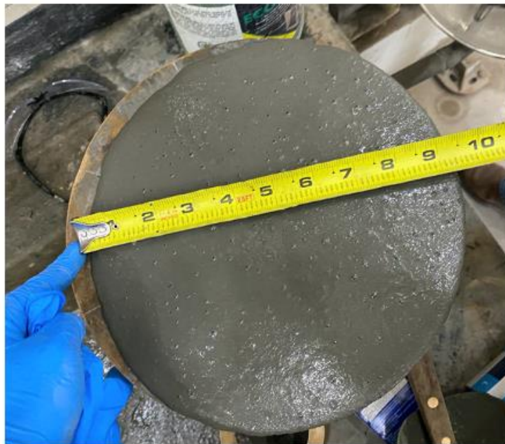
Figure 52. Photo. Flow diameter of 9-1/4 in. indicative of good workability.
