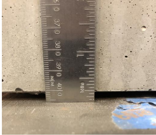
Figure 127. Photo. Underside of specimen N-6-5.75-B showing space between concrete and support.
