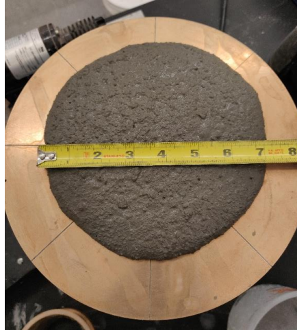
Figure 25. Photo. ASTM C1437 flow test.
