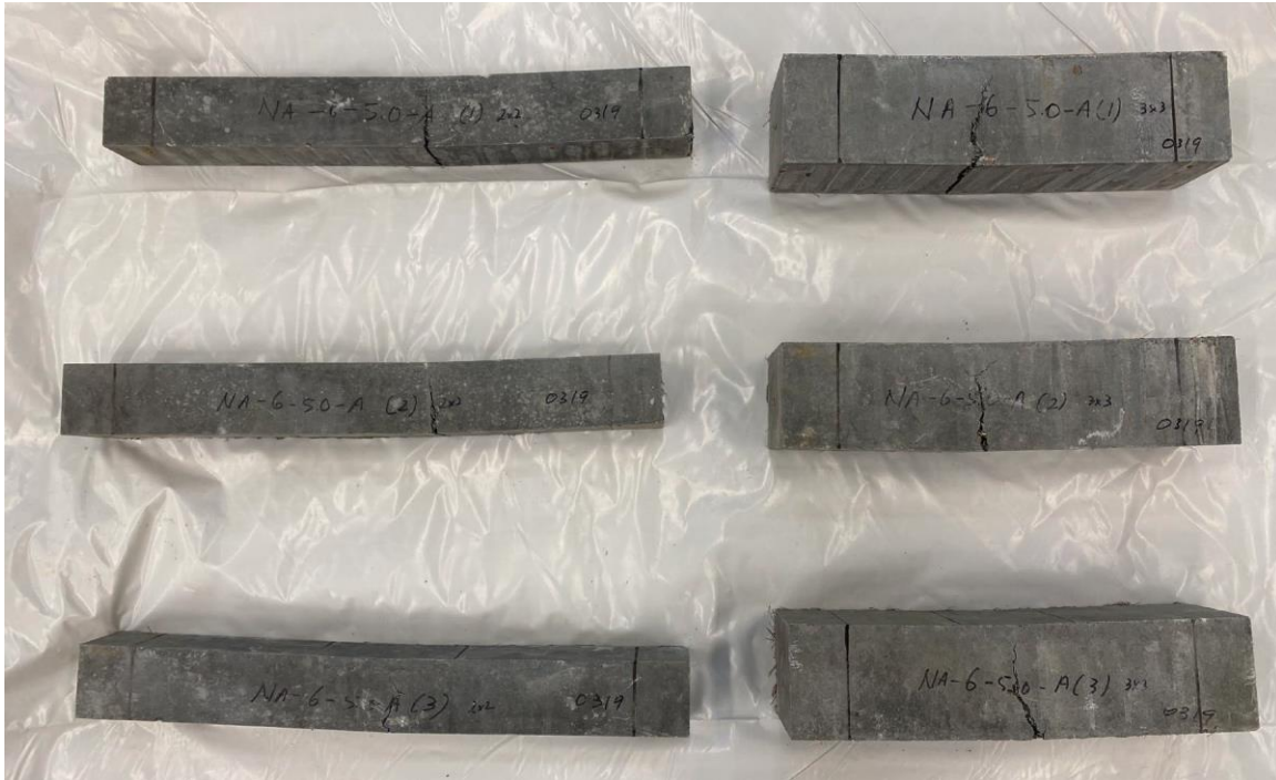
Figure 61. Photo. UHPC beam specimens after failure.
