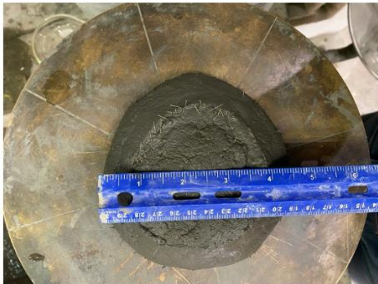
Figure 54. Photo. Flow diameter of 4-3/8 in. indicates poor workability of the above mix.
