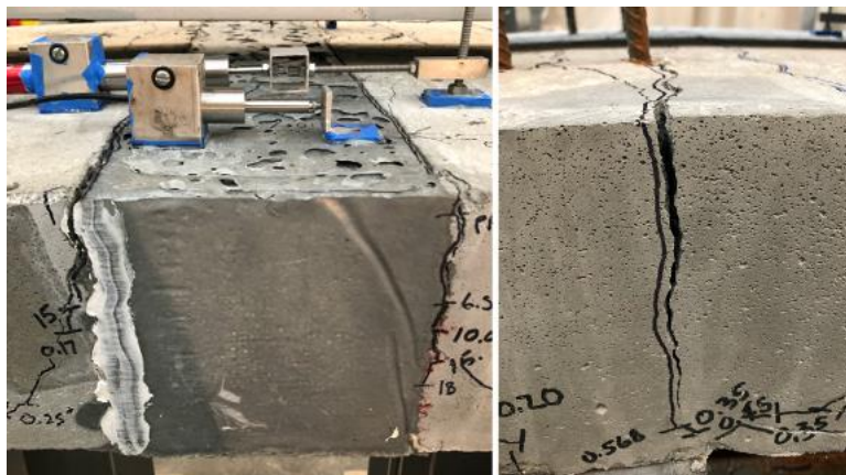
Figure 142. Photo. Specimen cracking at failure.
