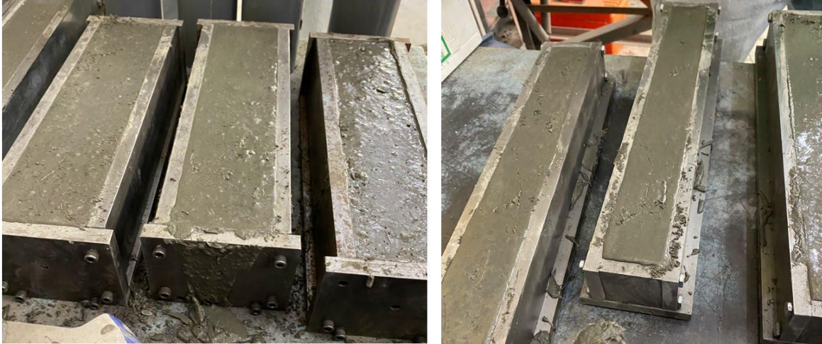
Figure 47. Photo. 3 in. by 3 in. by 12 in. molds (left) and 2 in. by 2 in. by 17 in. molds (right).
