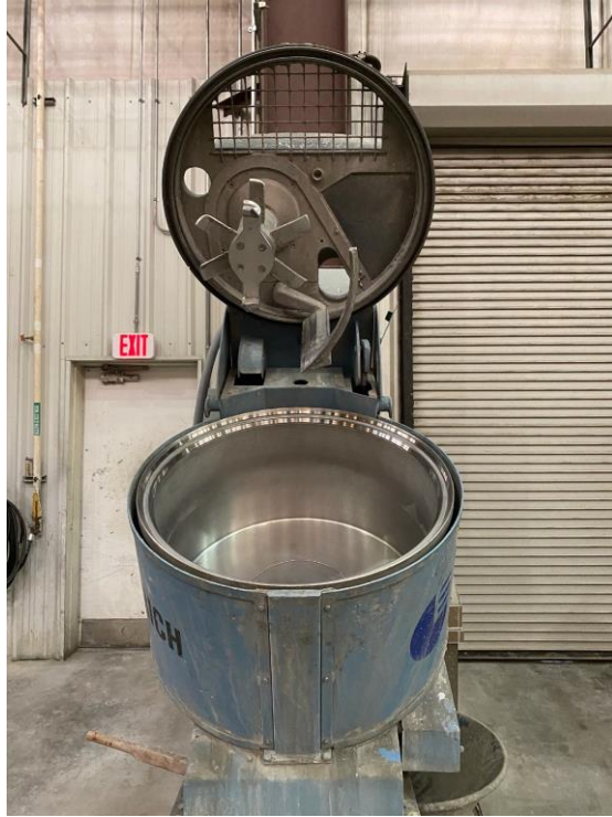
Figure 41. Photo. Eirich R08W used to make all UHPC in this investigation.
