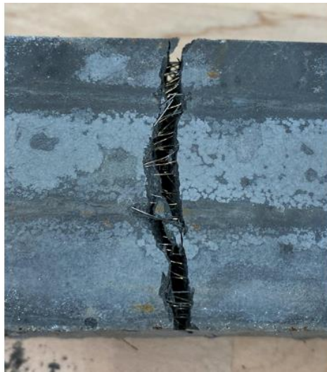
Figure 66. Photo. Close-up of the major crack that occurred in the 2 in. by 2 in. beam.
