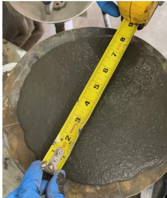
Figure 55. Photo. Flow test of 1F24Sf25.
