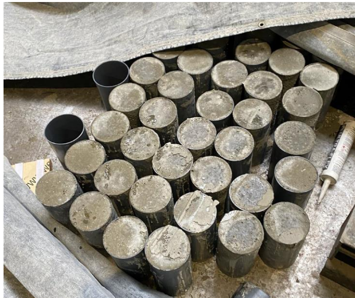
Figure 85. Photo. 4 in. by 8 in. cylinders cast to evaluate concrete strength.
