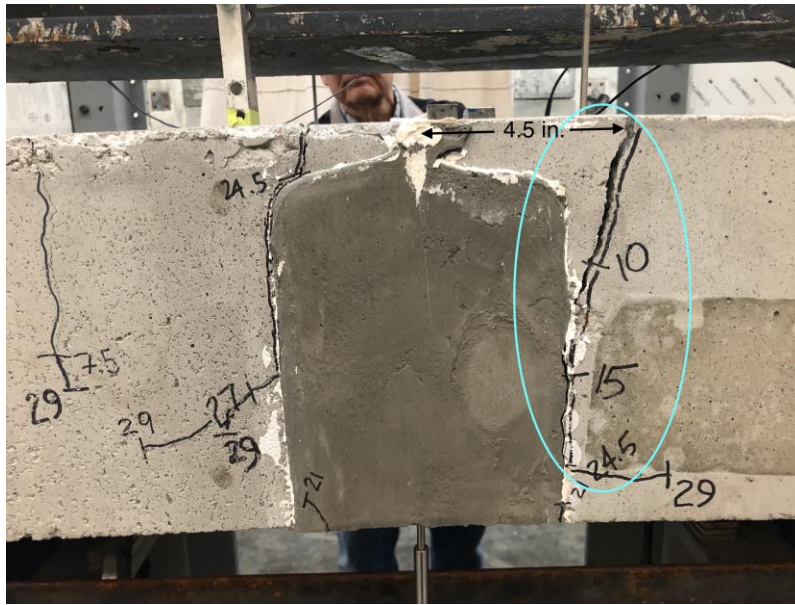
Figure 169. Photo. Cracking noted on south side of specimen.
