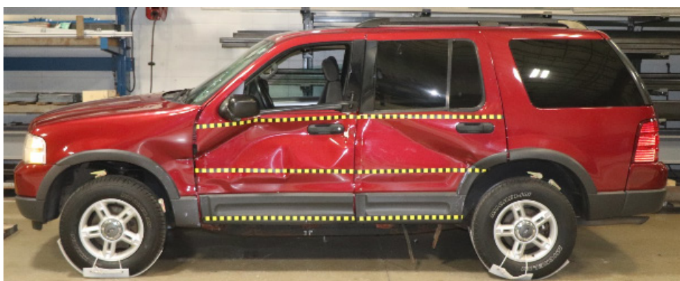
Figure 5-36 Impact Damage to the Explorer in Test 1 Where Inch Tape Measurements Were Made
