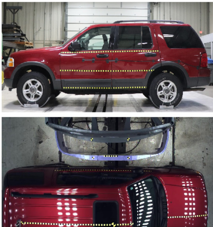
Figure 5-14 Markers on the Exterior of the 2003 Explorer in Test 1
