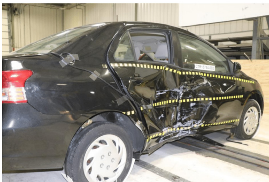
Figure 5-50 Yaris Deformations Compared with Simulated Response
