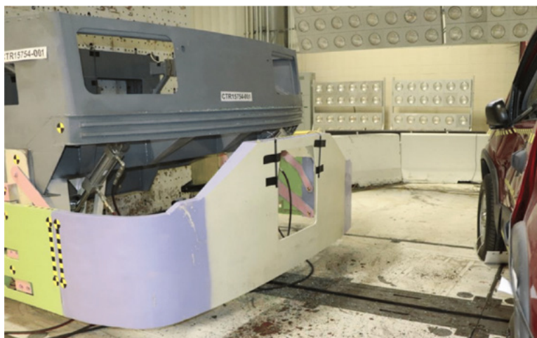
Figure 5-33 Front Enclosure Post-Test 1
