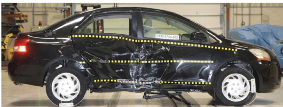
Figure 5-46 Impact Damage to the Yaris in Test 2 Where Inch Tape Measurements Were Made
