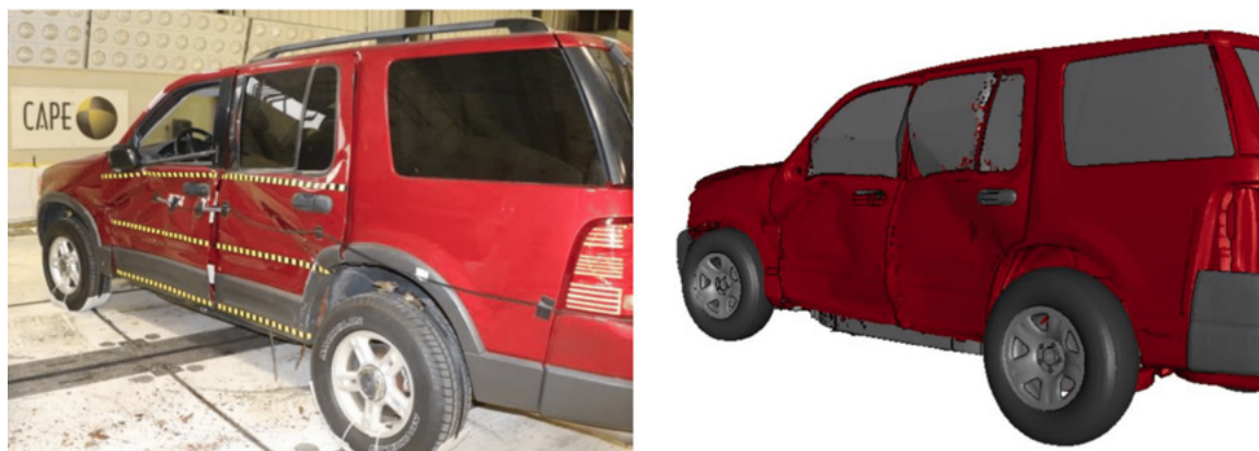
Figure 5-40 Explorer Deformations Compared with Simulated Response
