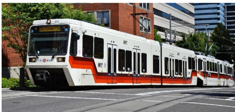
Figure 2-3 Portland SD660 Operating on Shared Right-of-Way (photographed by Steve Morgan)
