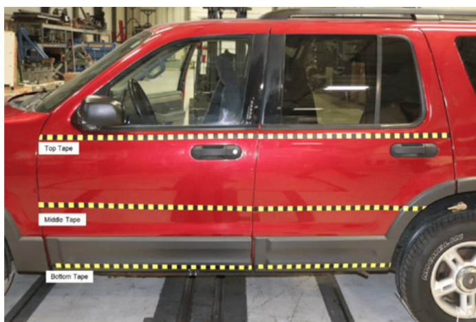
Figure 5-34 Location of Inch Tape on the 2003 Ford Explorer (pre-test)
