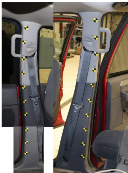
Figure 5-15 B-Pillar Deformation Measurement Locations Pre-crash (left two images are driver side, right image is passenger side)
