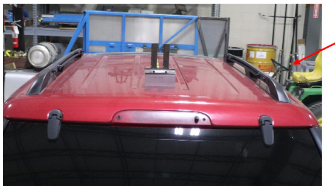
Figure 5-10 Test 1 Forks for Laser Speed Trap Measurements
