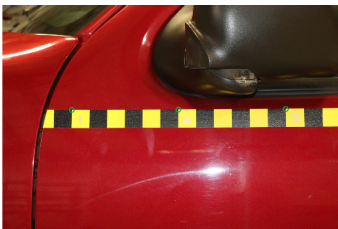
Figure 5-35 Location of Inch Tape Measurements with the Laser (Test 1)
