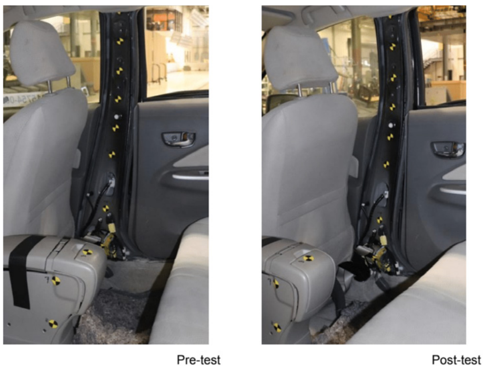
Figure 5-51 B-Pillar Deformation in the Yaris
