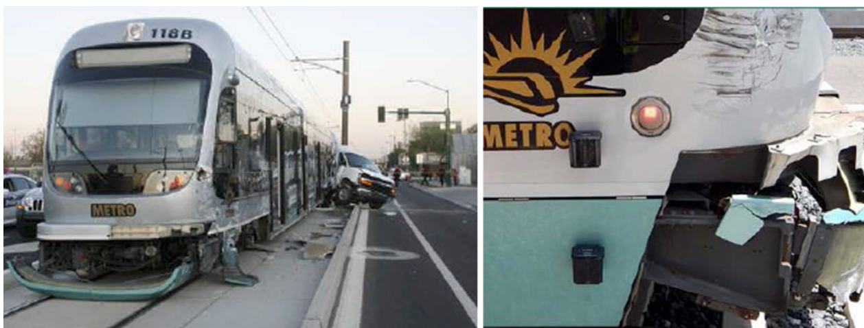
Figure 6-2 Example of Damage to the Front Enclosure of the KI LRV After Impact with an Automobile [8]
