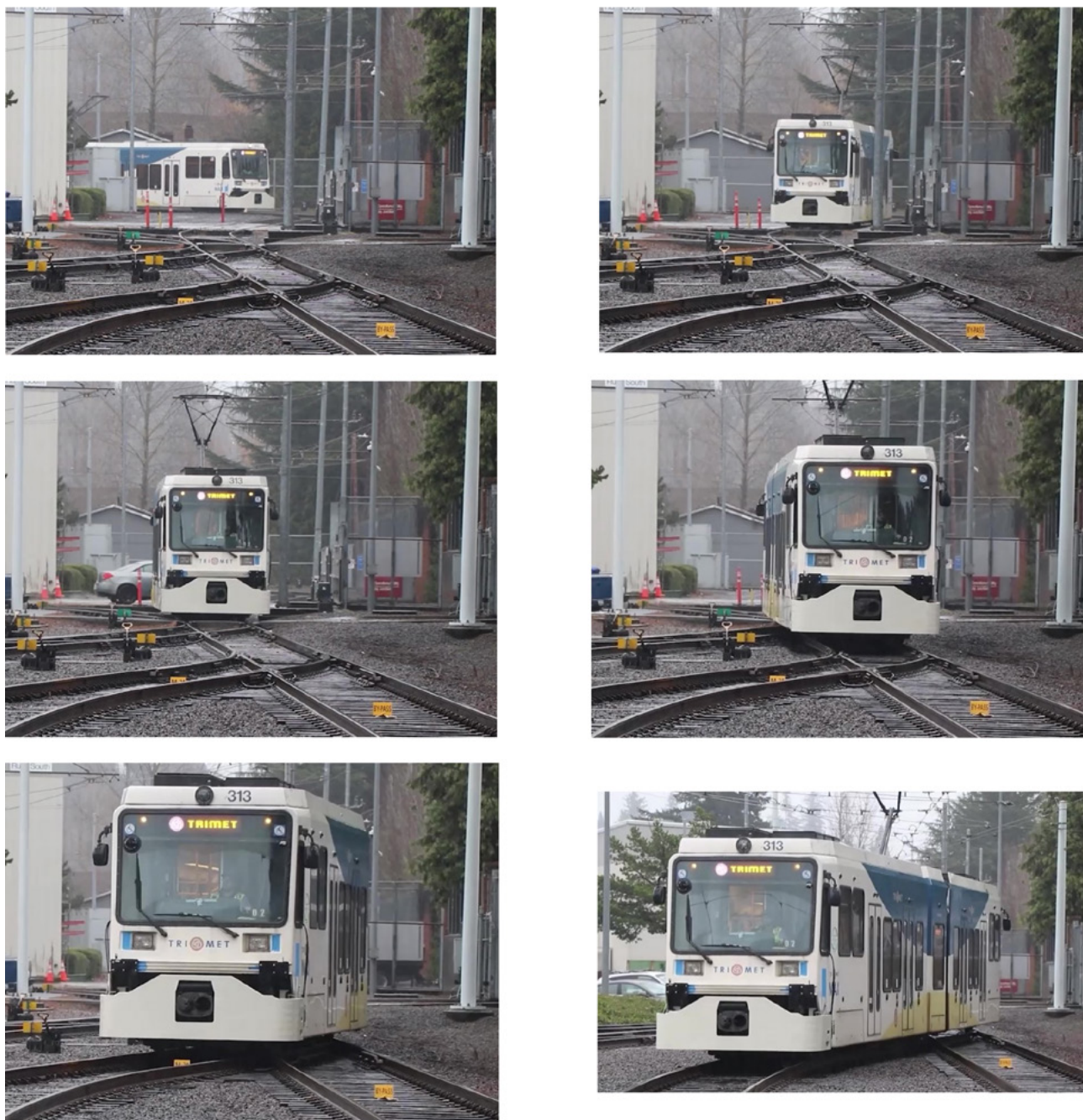
Figure 4-5 Type 3 Ride Test with a Temporary Front Enclosure Retrofit
