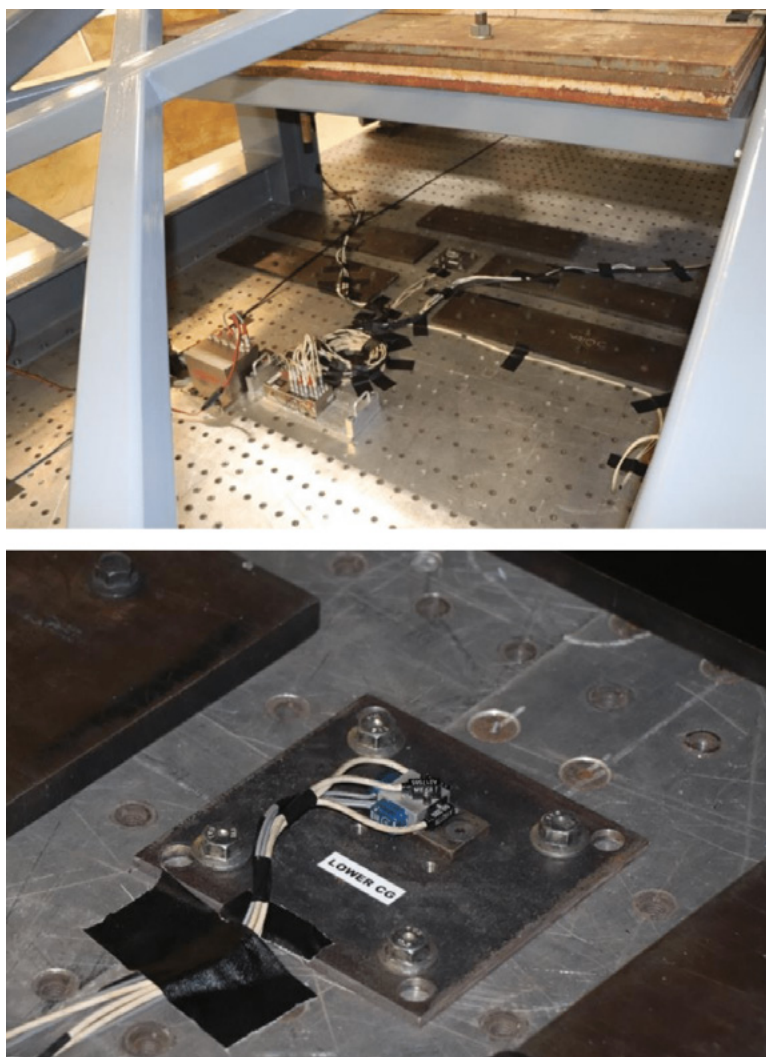
Figure 5-28 Test 3 Accelerometers Mounted to the Test Sled
