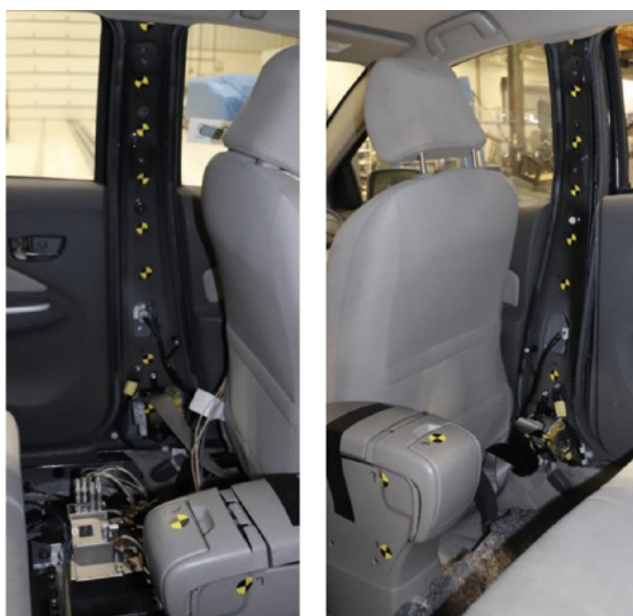
Figure 5-24 B-Pillar Deformation Measurement Locations Pre-test in Test 2
