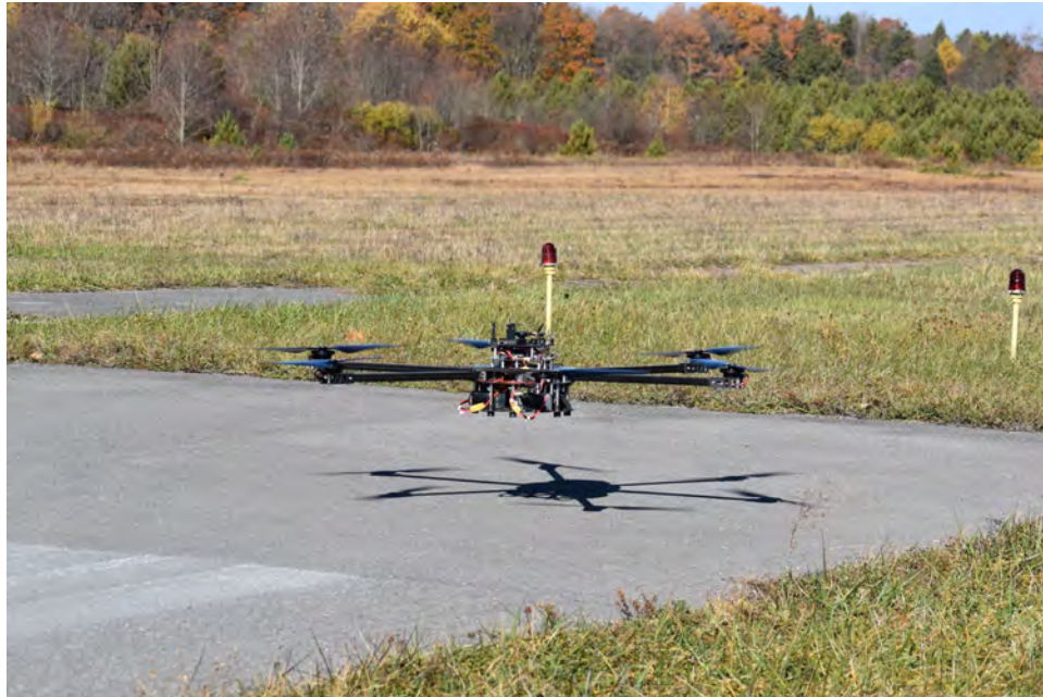
Figure 22. Full-size reconfigurable unmanned aircraft system (hexacopter configuration) in the landing procedure after one mission.
