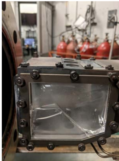
Figure 4. Liner deformation and broken windows due to compressive failure at high temperature.
