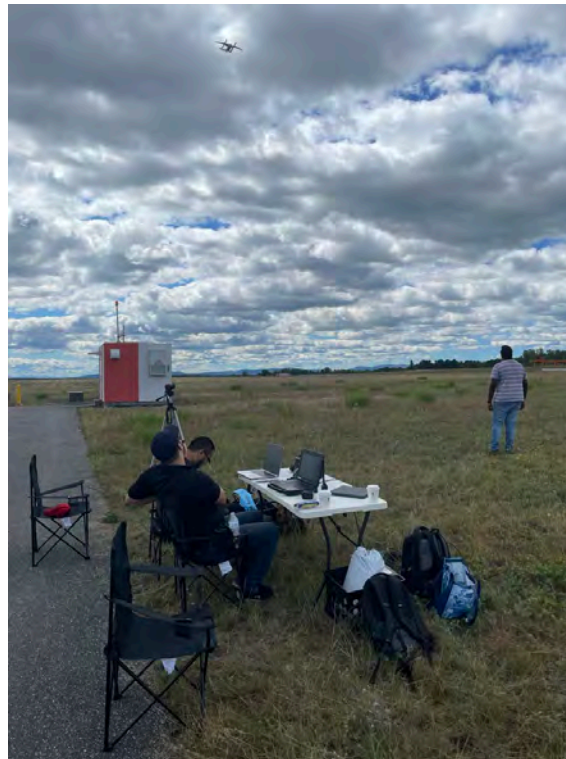
Figure 25. Noise measurement of the ALIA-250 in flyover by the Penn State team.
