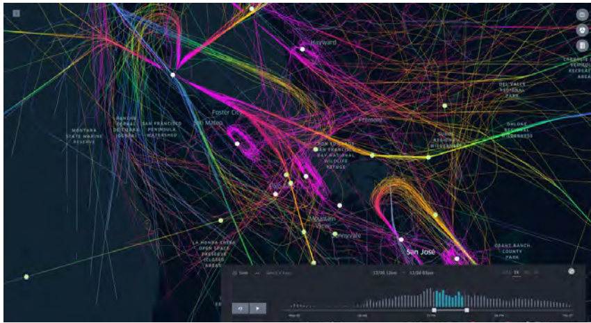
Figure 1. MONA visualization using kepler.gl (n.d.) and deck.gl (n.d.) of traffic patterns in the San Francisco Bay Area, including a 24-hr view of aircraft traffic patterns. Trajectories are colored by altitude, with purple/magenta indicating low altitudes and blue indicating high altitudes.
