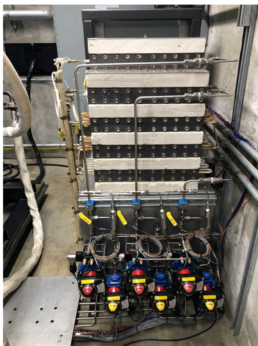
Figure 3. Photograph of the assembled fuel heating system.
