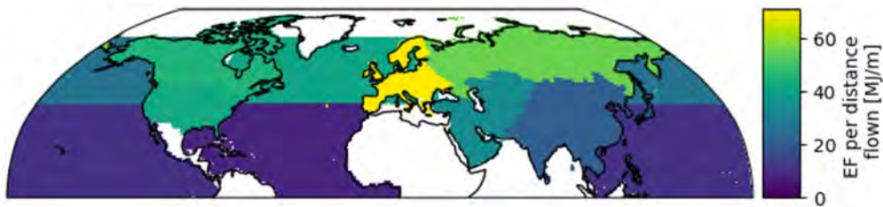
Figure 19. Spatial distribution of mean contrail energy forcing (EF) per distance flown in the Northern Hemisphere (Agarwal 2021).
