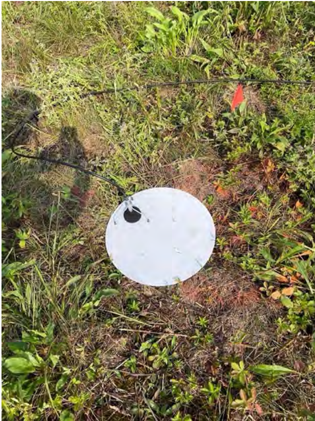
Figure 18. Inverted ground-plane (left) and elevated (right) microphone installations.
