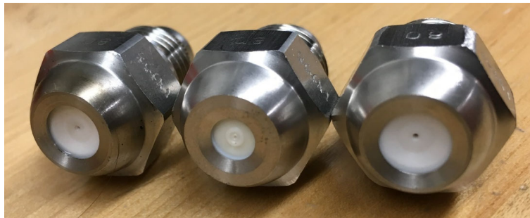
Figure 3. Nozzles tested during lean blowout testing in the M1 combustor.
