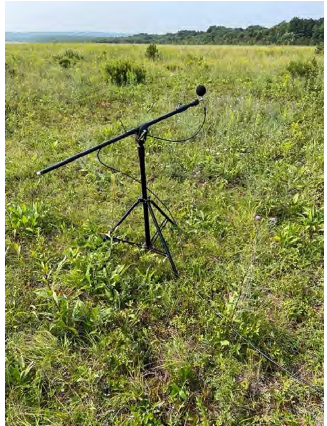
Figure 18. Inverted ground-plane (left) and elevated (right) microphone installations.
