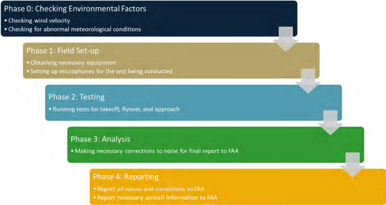
Figure A1. Overview of the noise certification process as described in Parts 21 and 36 and Advisory Circular 36-4D.
