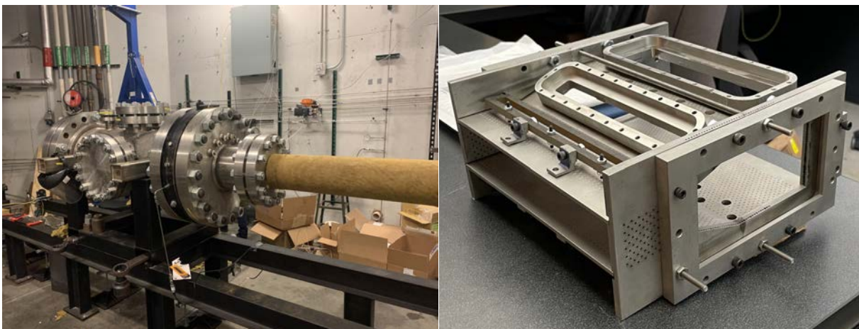
Figure 8. Photograph of the high-pressure system (left) and combustor frame (right).
