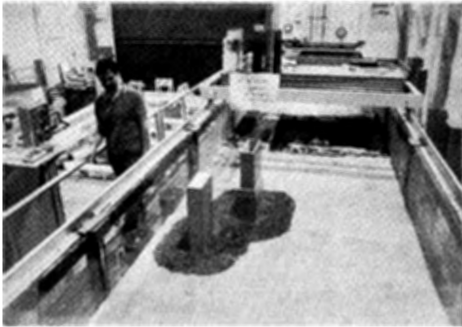
Figure 17. Riprap experiment before flume operation.
