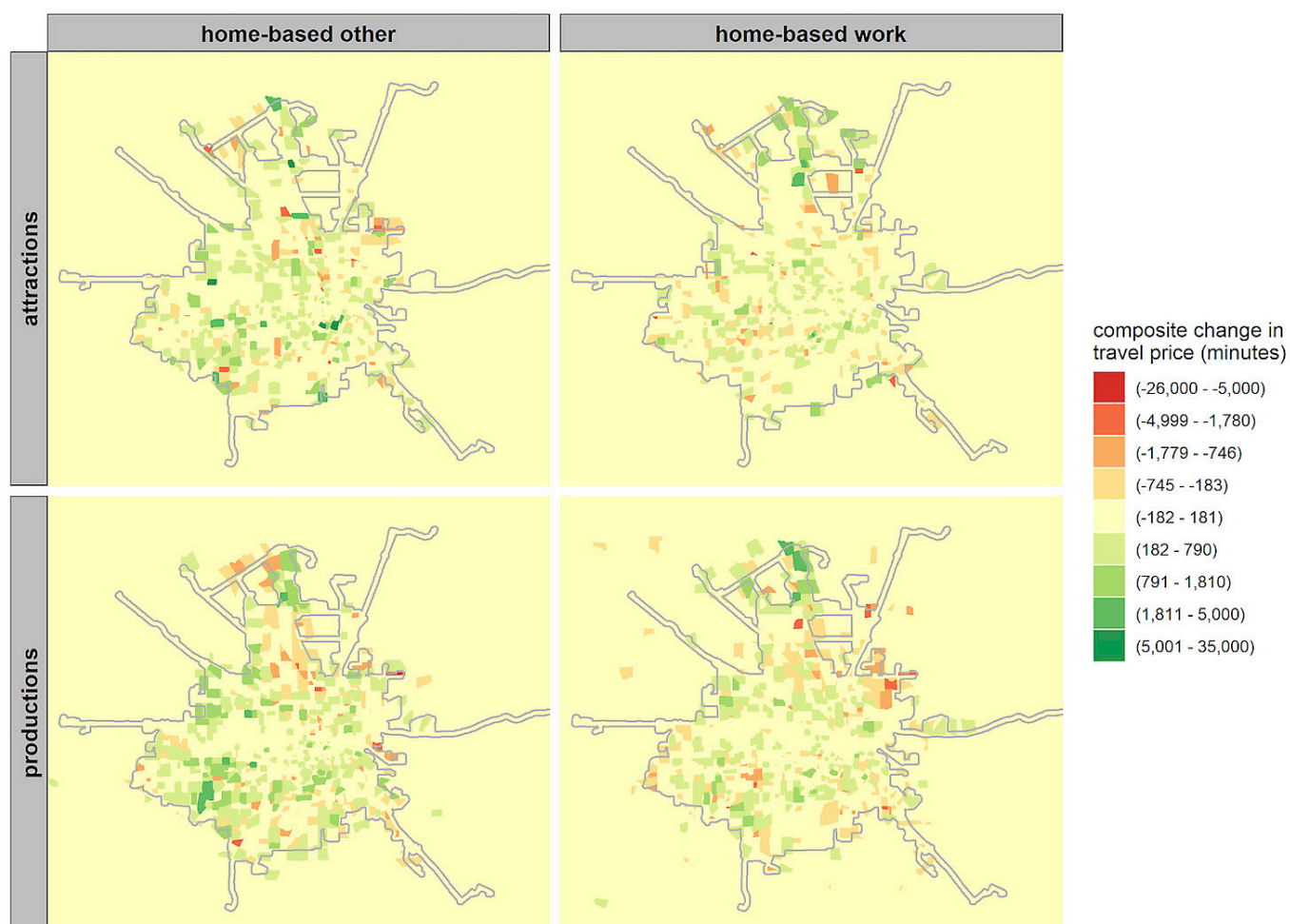
Figure 1-1 Weekday user benefits resulting from a major bus network redesign in Houston, TX, calculated using FTA's STOPS model and Summit software
