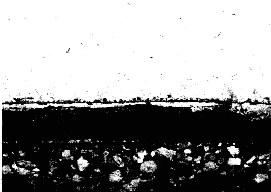
Figure 92. Moderate surface type corrosion.
