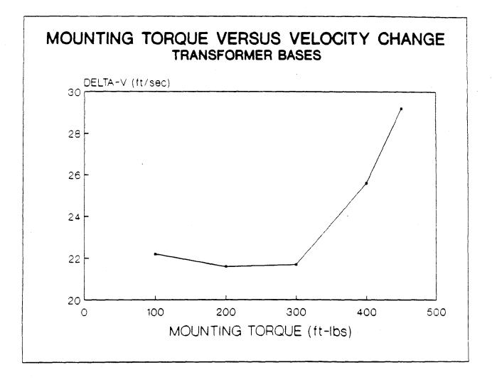
Figure 4. Change in velocity versus mounting torque.
