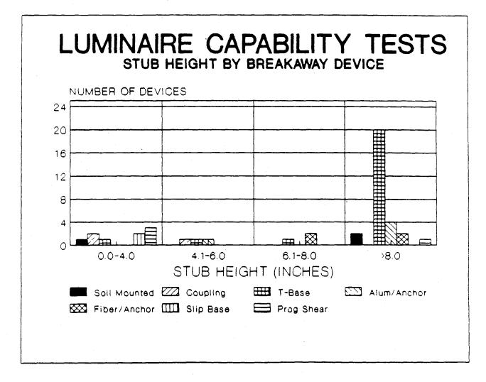
Figure 2. Distribution of stub height by breakaway device.
