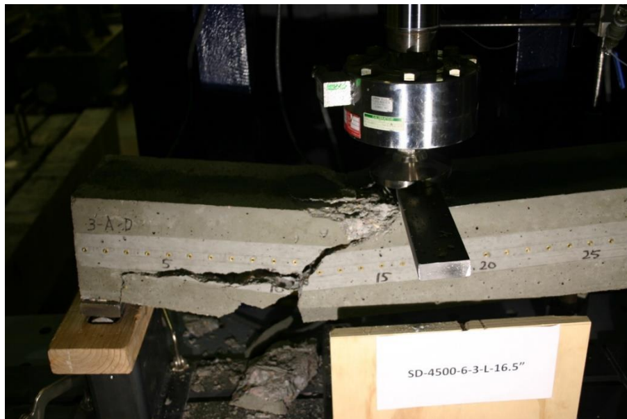
Figure 394 Picture of Failed Prism for SD-4500-6-3-L
