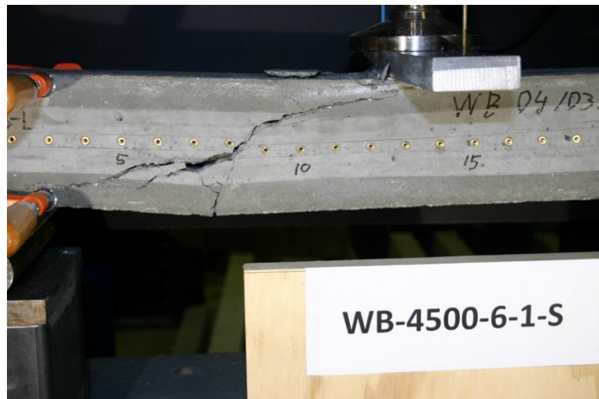
Figure 123 Picture of Failed Prism WB-4500-6-1-S
