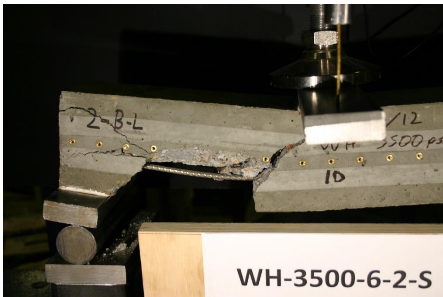
Figure 358 Picture of Failed Prism for WH-3500-6-2-S
