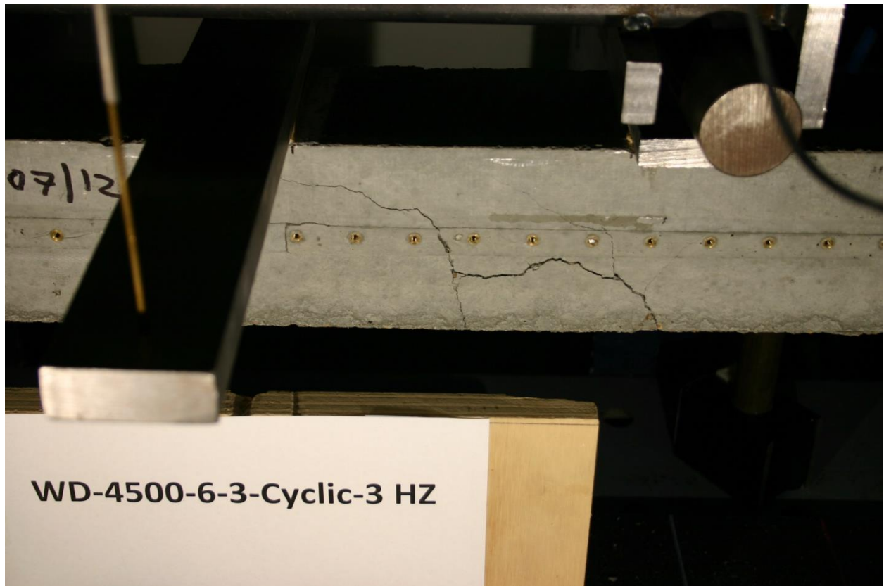
Figure 67. Prism made with WD wire failed at 162,760th cycle of loading
