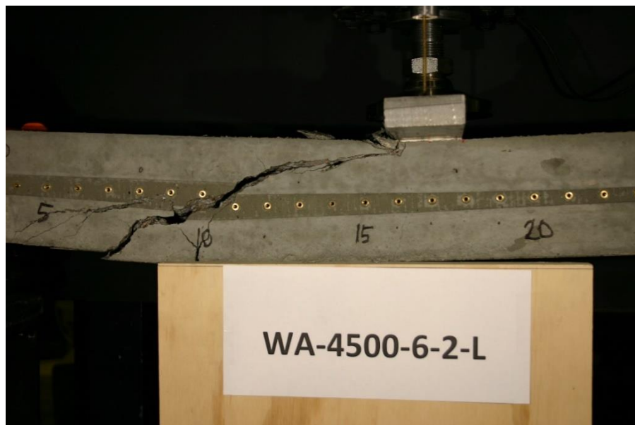
Figure 117 Picture of Failed Prism WA-4500-6-2-L
