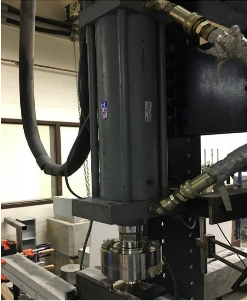
Figure 29. Actuator used for conducting load tests on prisms containing strands
