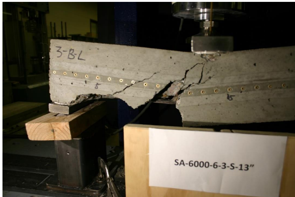
Figure 462 Picture of Failed Prism for SA-6000-6-3-S
