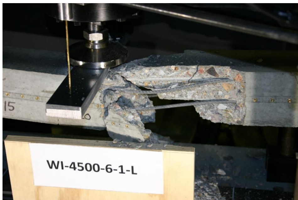
Figure 177 Picture of Failed Prism WI-4500-6-1-L
