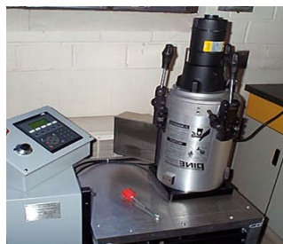
b) Compacting using the Gyratory Compactor
