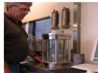
f) Testing in temperature-controlled chamber
