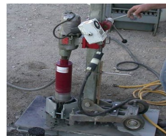
c) Coring sample to 100-mm diameter
