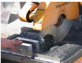
d) Cutting sample to 100-mm high
