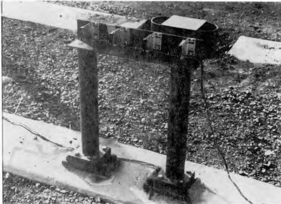
Figure 9. Speed trap system mounted at the pendulum site.
