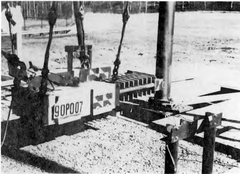
Figure 11. Typical slip base luminaire support.
