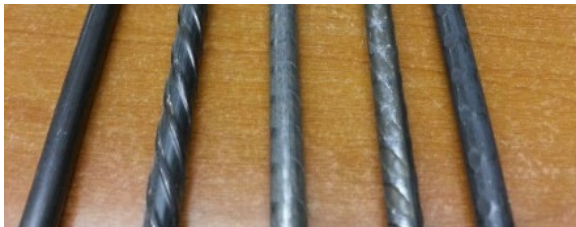
Figure 1: Five 5.32 mm diameter wires with different indentation types
