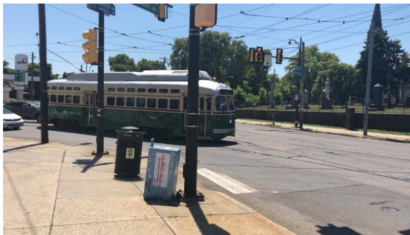
Figure 63: Center of trolley encroaching inside lane
