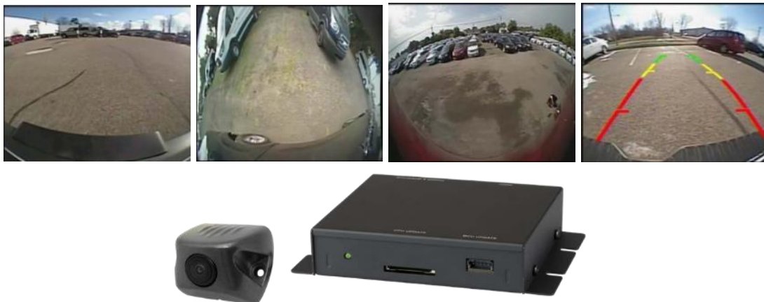
Figure 75: SEON's inView 360 Collision Avoidance System 2
