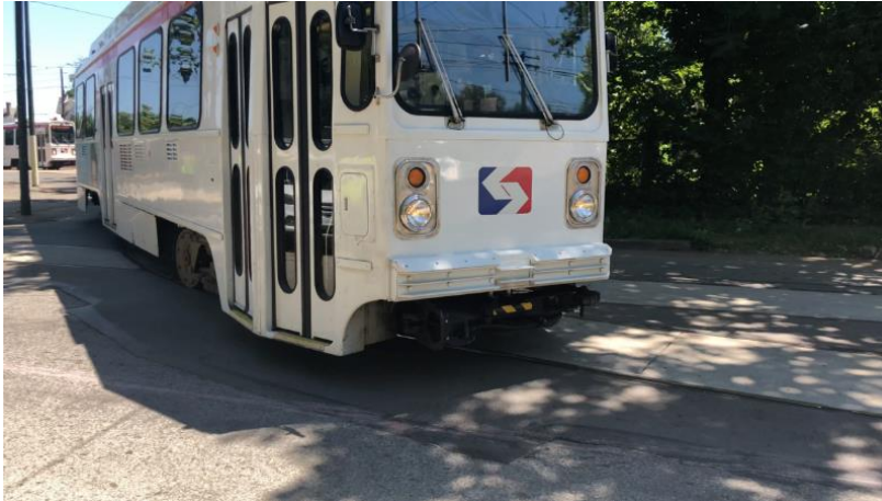
Figure 62: Corner of trolley swinging out in curve
