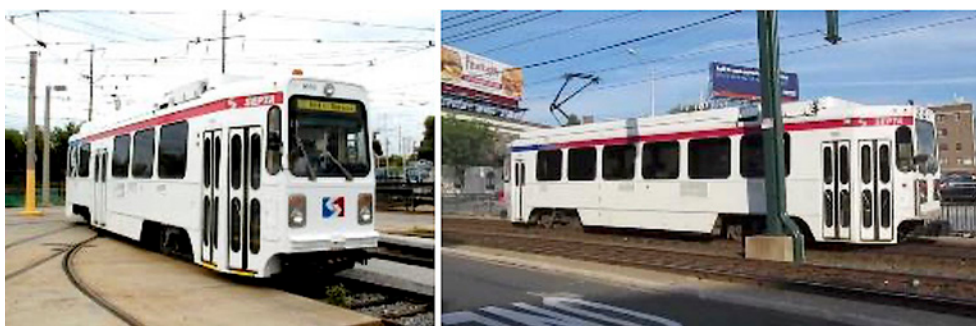
Figure 3-61 Kawasaki Heavy Industries single-ended (left) and double-ended (right) cars
