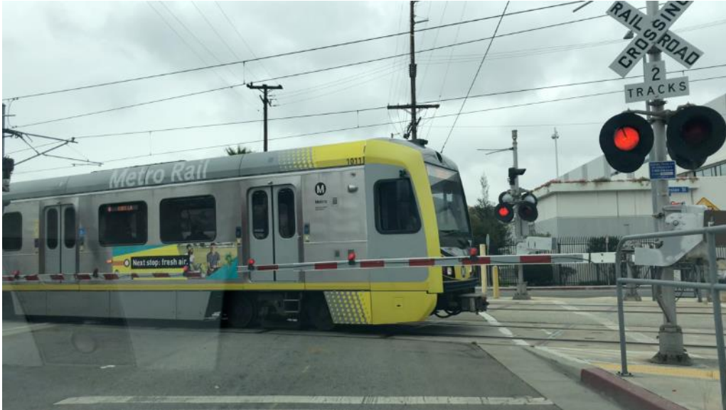
Figure 47: Four-quadrant gated crossing
