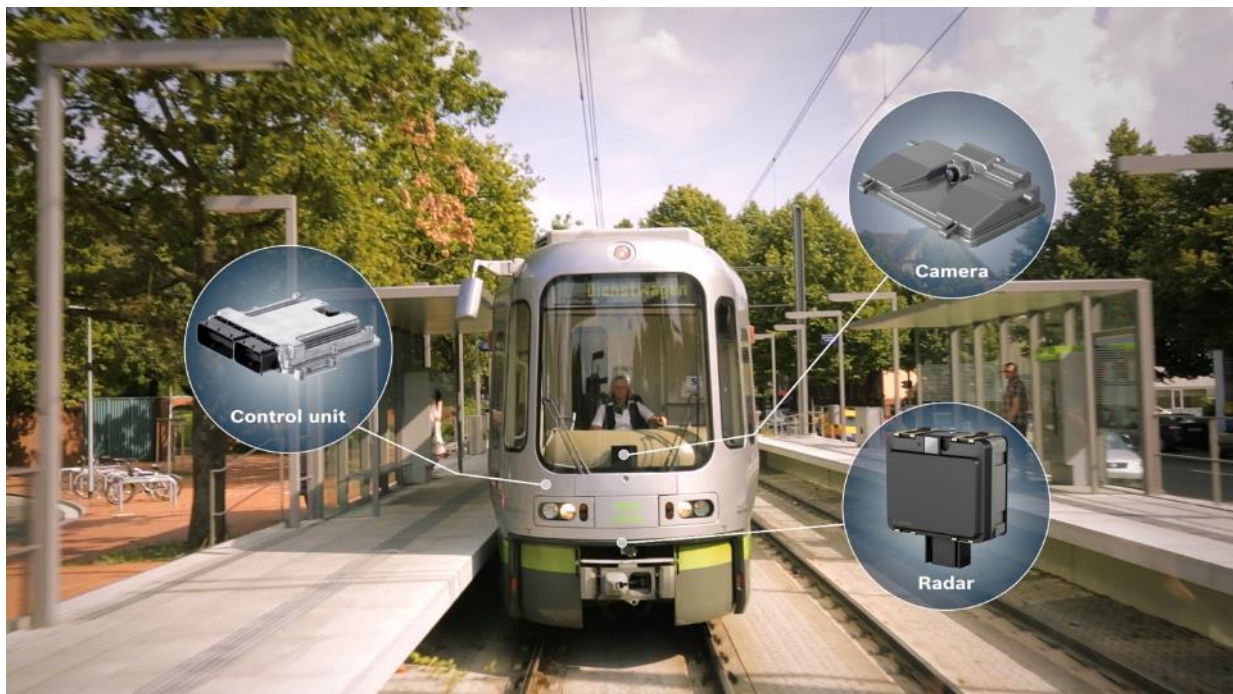
Figure 2: Bosch Engineering Tram forward collision warning system
