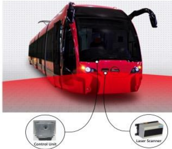
Figure 4: “Silkworm” with collision avoidance system
