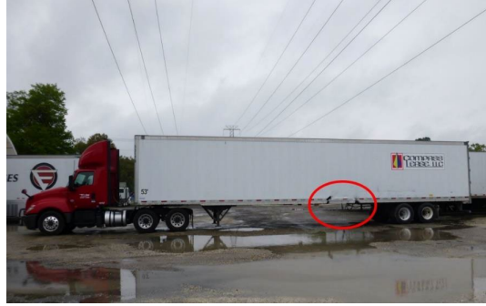
Figure B.7. Left Side of Combination Vehicle. Damage to Lower Edge of Semitrailer Sidewall Rails Is Circled in Red
