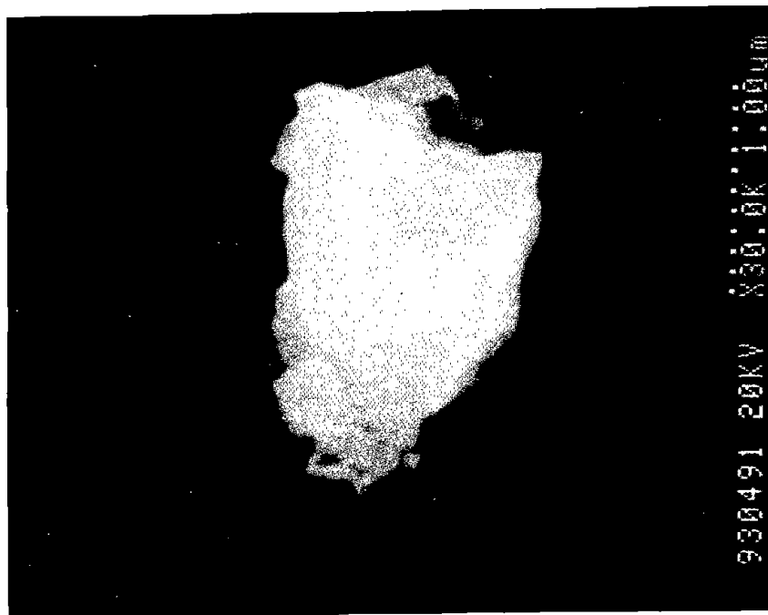
Figure 37. EDX analysis and SEM micrograph of 1- \mu m particle collected on filter within confinement zone during blasting.
