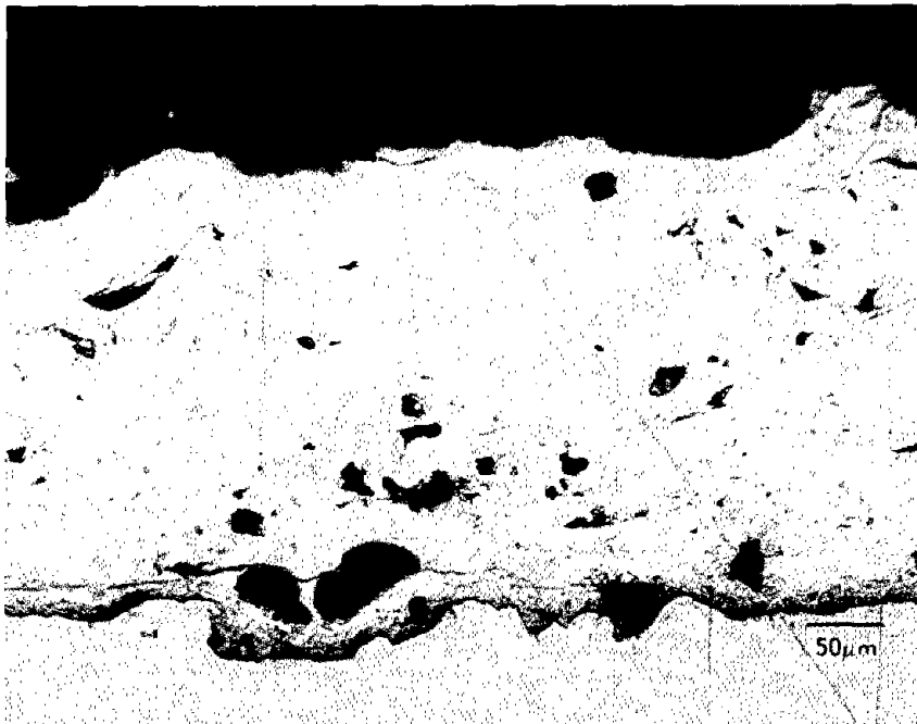
Figure 61. Thermally sprayed 85/15 zinc/aluminum alloy.
