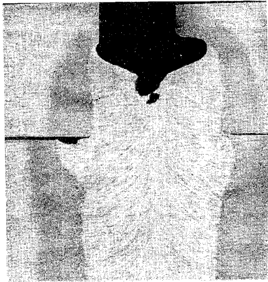
Figure 10. Weld centerline slag inclusion in a run-off block.
