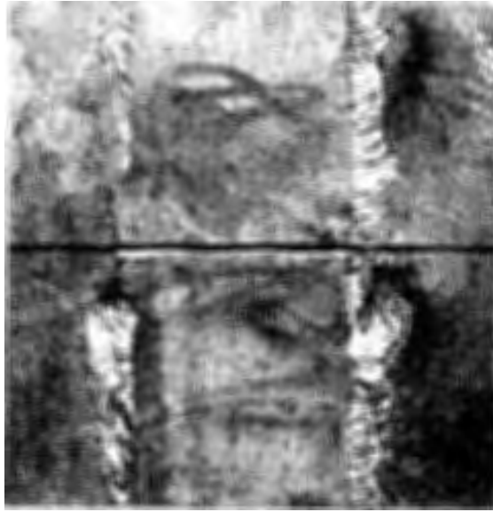
(a) Weld surface indication.
