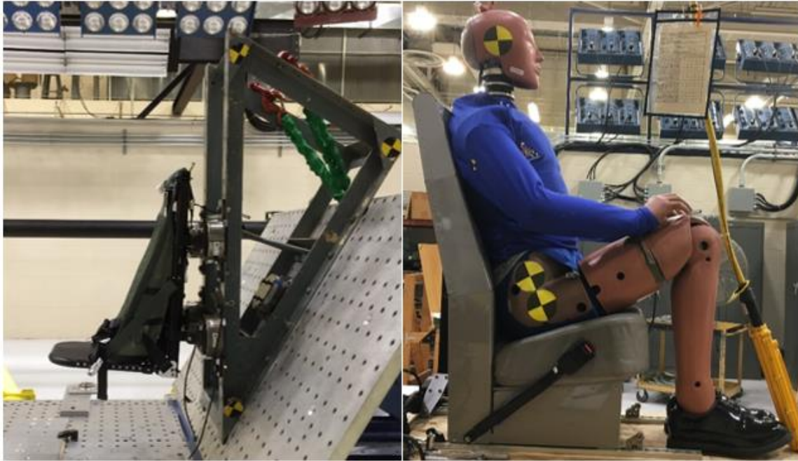
Figure 4: Bulkhead-mounted seat (left) and floor-mounted seat (right) in the configuration for 1-G seating procedure
