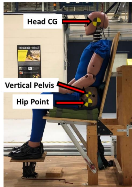
Figure 5: FAA Hybrid III on wooden 1-G seating fixture
