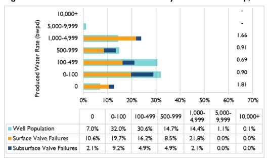
Figure 19: SPPE Failures and Active Wells by Water Rate Group, 2021
