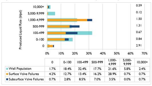
Figure 21: SPPE Failures and Active Wells by Total Liquid Rate, 2021
