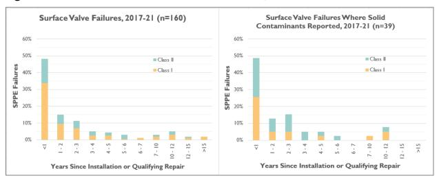
Figure 32: Time to Failure and Valve Service Class, 2017-2021
