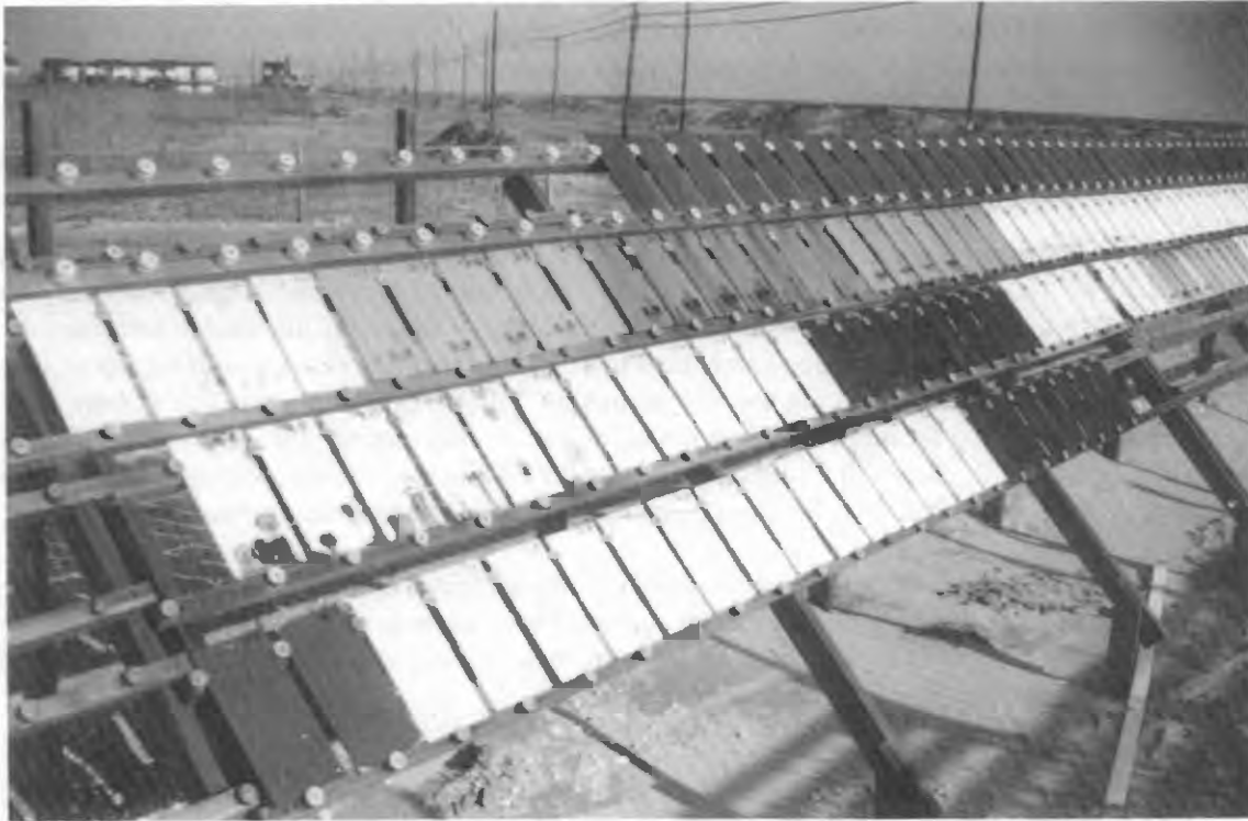
Figure 1. Panels exposed at Sea Isle City test site after approximately 18 months of exposure.
