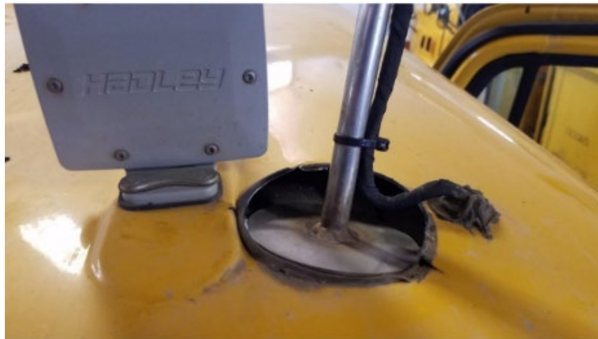
Figure 22. NYC Antenna Installation on a City vehicle.
