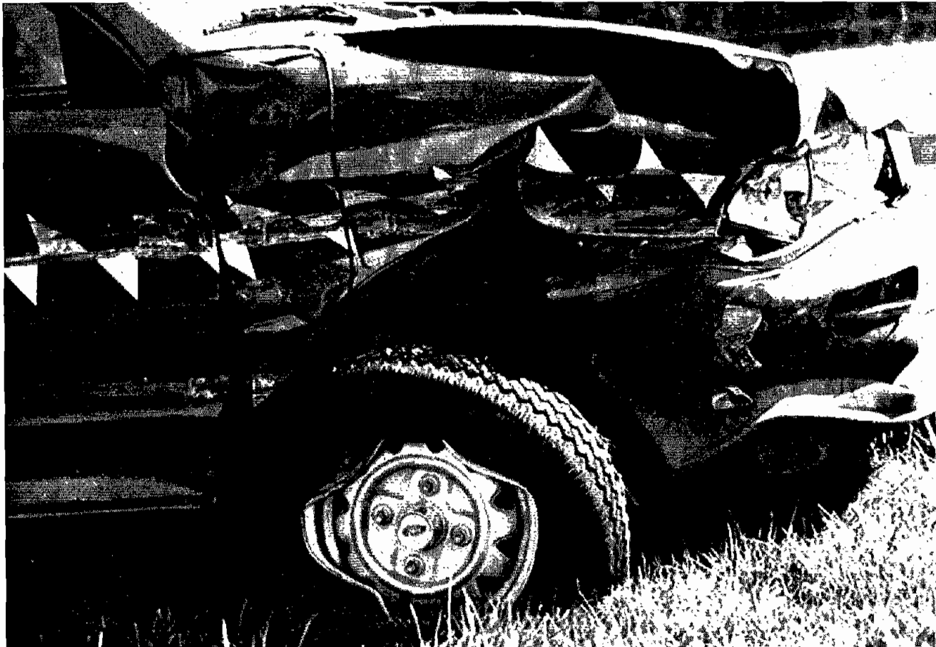
Figure 40 Typical impact damage to the sheet-metal of a small car after a guardrail test.
